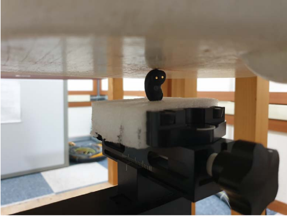
SAR Test Picture(Top), Test separation distance : 0 mm
