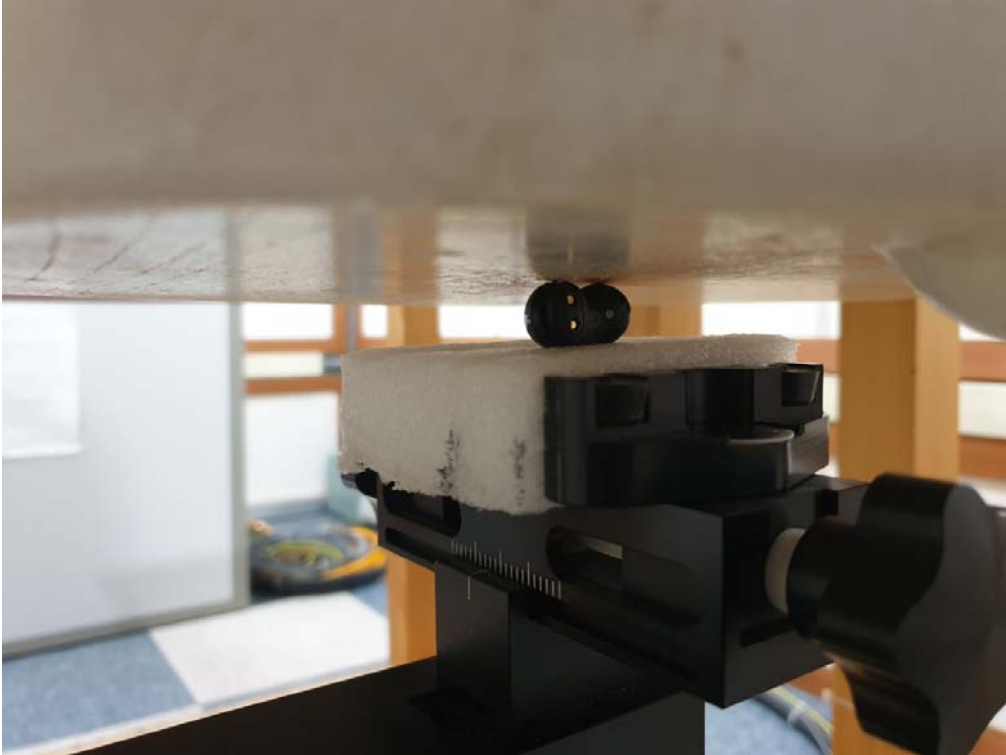
SAR Test Picture(Right), Test separation distance : 0 mm
