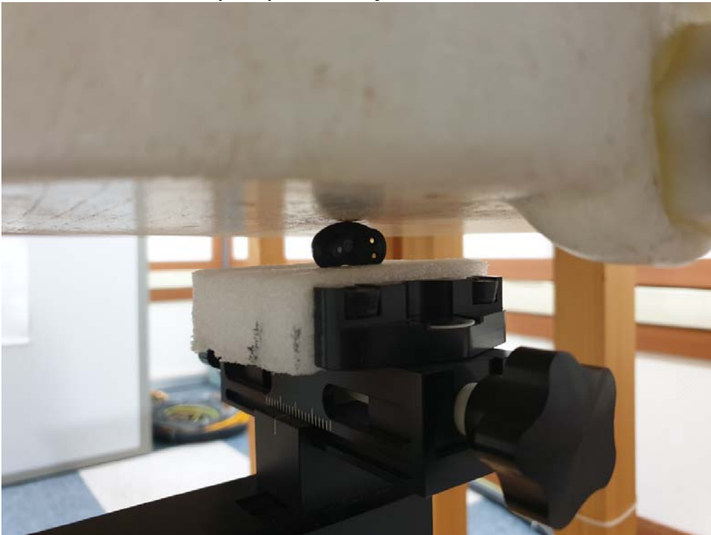
SAR Test Picture(Left), Test separation distance : 0 mm
