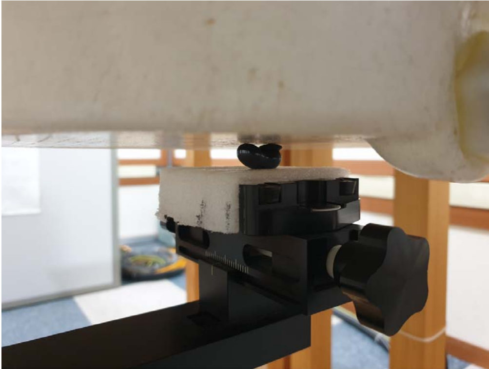
SAR Test Picture(Front), Test separation distance : 0 mm
