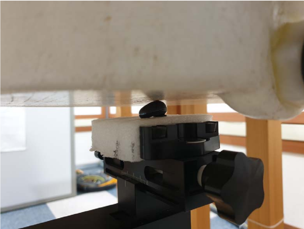
SAR Test Picture(Back), Test separation distance : 0 mm
