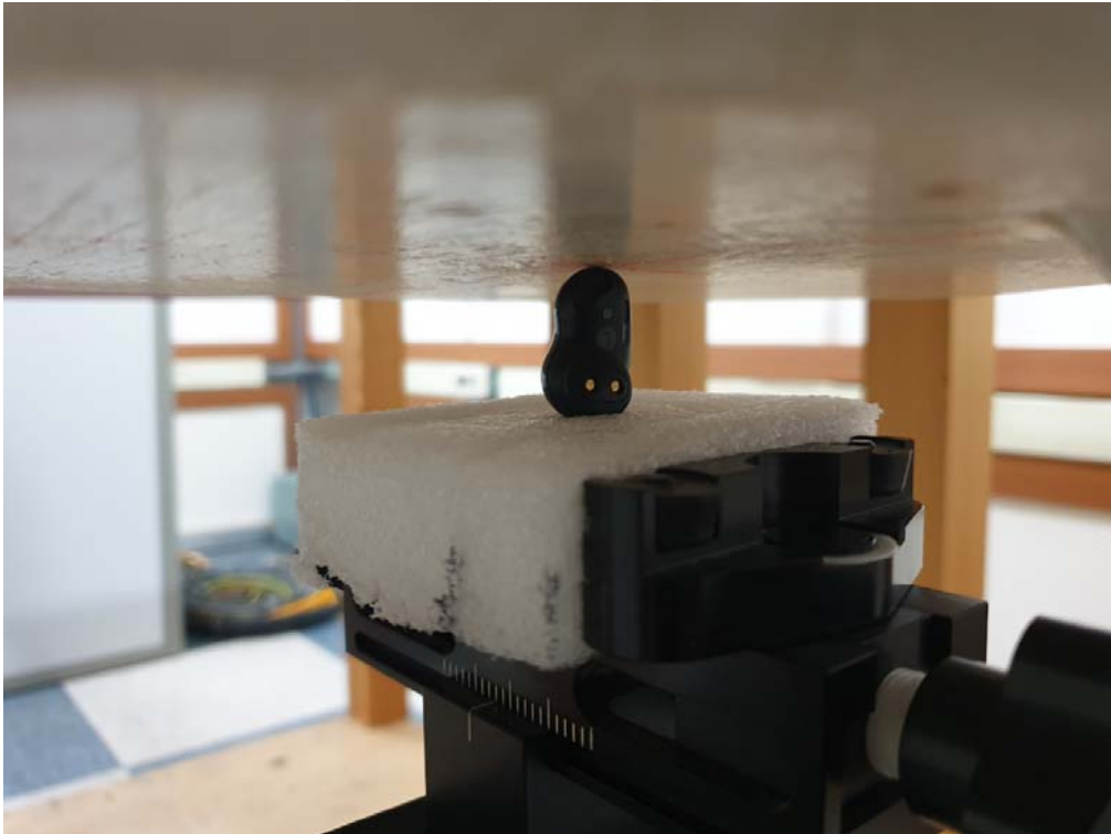
SAR Test Picture(Bottom), Test separation distance : 0 mm
