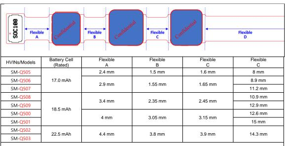
Except for differences in battery capacity and plexible area length, the circuitry and components/placement and RF characteristics are identical.
