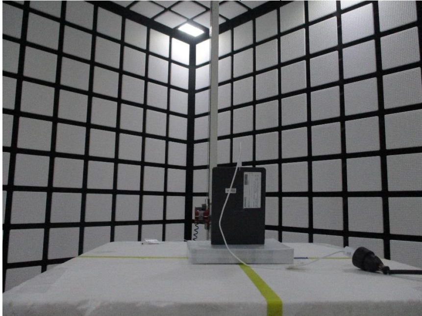
ABOVE 1 GHz REAR TEST PHOTO(Z axis)
