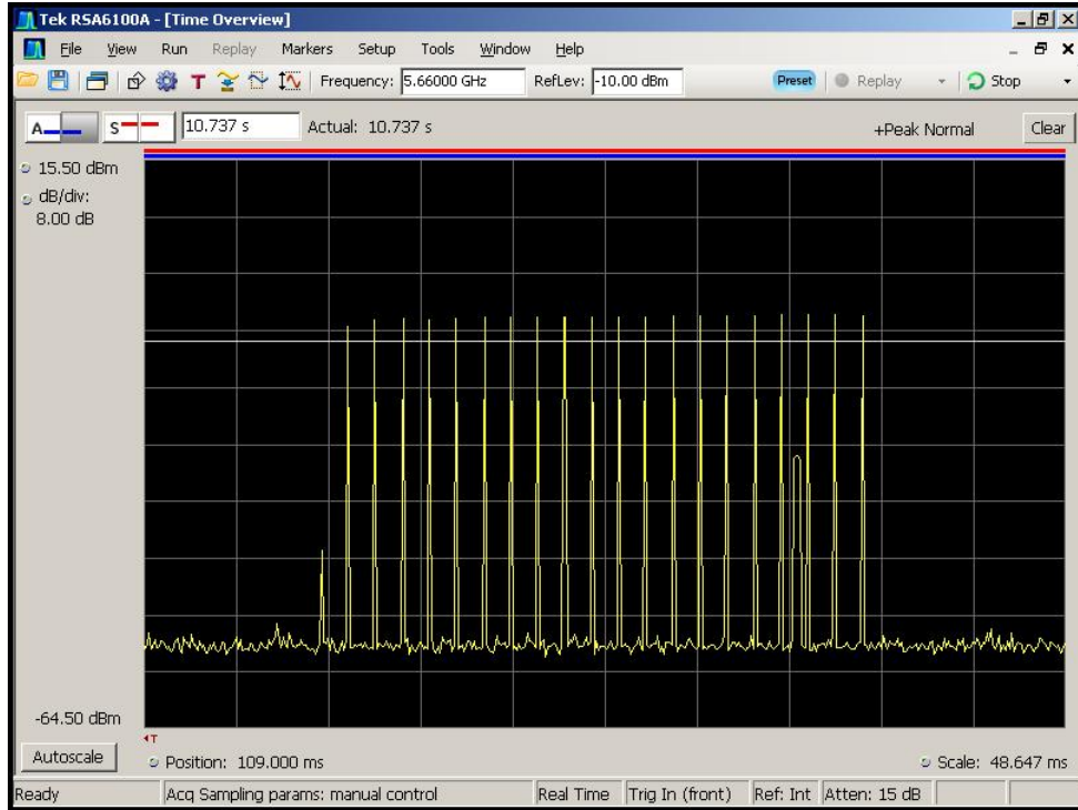
Figure 6-1. Type 1 Radar Pulse
