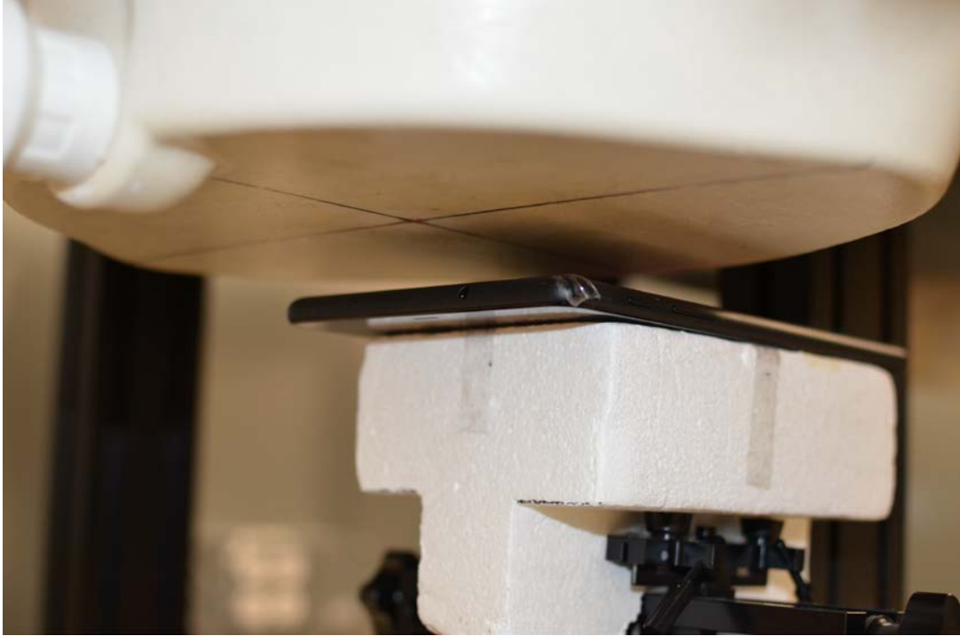
SAR Test Setup Photo 5: Back Side at 1.9 cm
