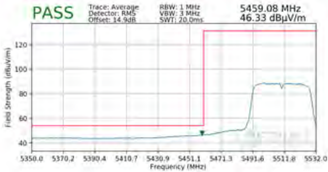
Plot 7-95. Radiated Lower Band Edge Plot SISO ANT1 (Average – UNII Band 2C)
