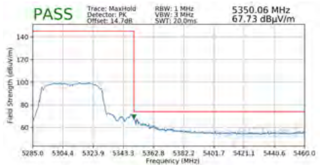
Plot 7-94. Radiated Upper Band Edge Plot SISO ANT1 (Peak – UNII Band 2A)
