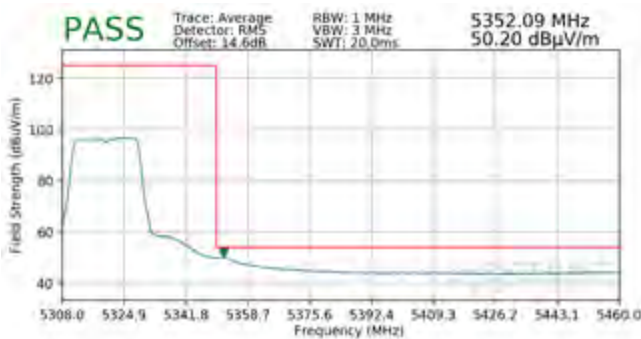
Plot 7-86. Radiated Upper Band Edge Plot SISO ANT1 (Average – UNII Band 2A)
