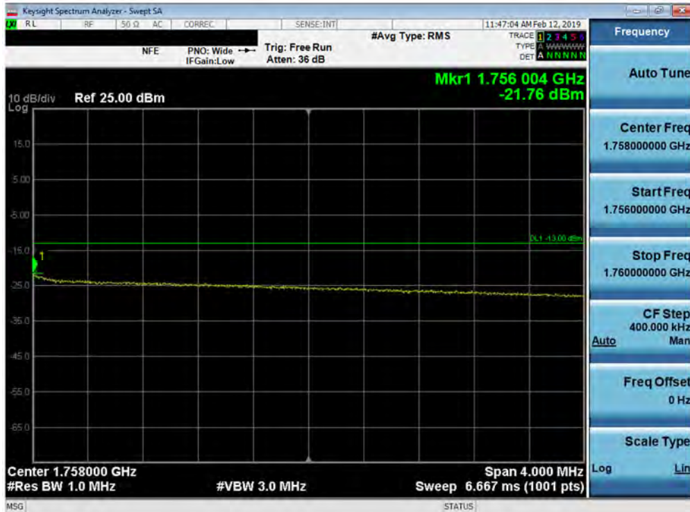
Plot 7-133. Upper Extended Band Edge Plot (Band 4 - 10.0MHz QPSK - Full RB Configuration)
