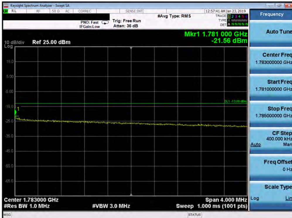
Plot 7-135. Upper Extended Band Edge Plot (Band 66 - 10.0MHz QPSK - Full RB Configuration)
