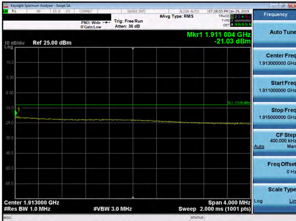
Plot 7-167. Upper Extended Band Edge Plot (Band 2 - 15.0MHz QPSK - Full RB Configuration)
