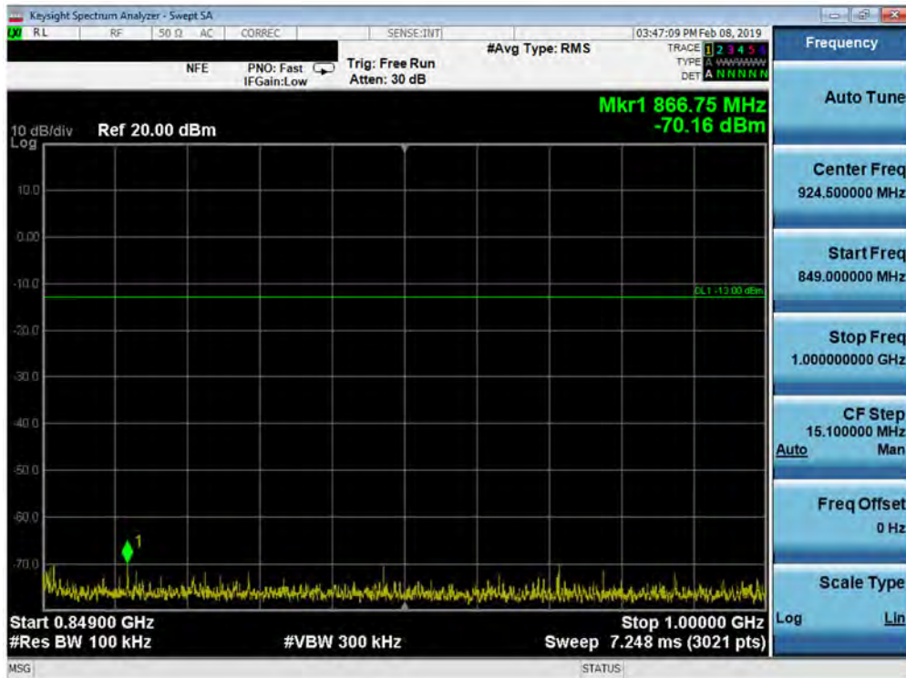
Plot 7-59. Conducted Spurious Plot (Band 5 - 10.0MHz QPSK - RB Size 1, RB Offset 0 - Low Channel)
