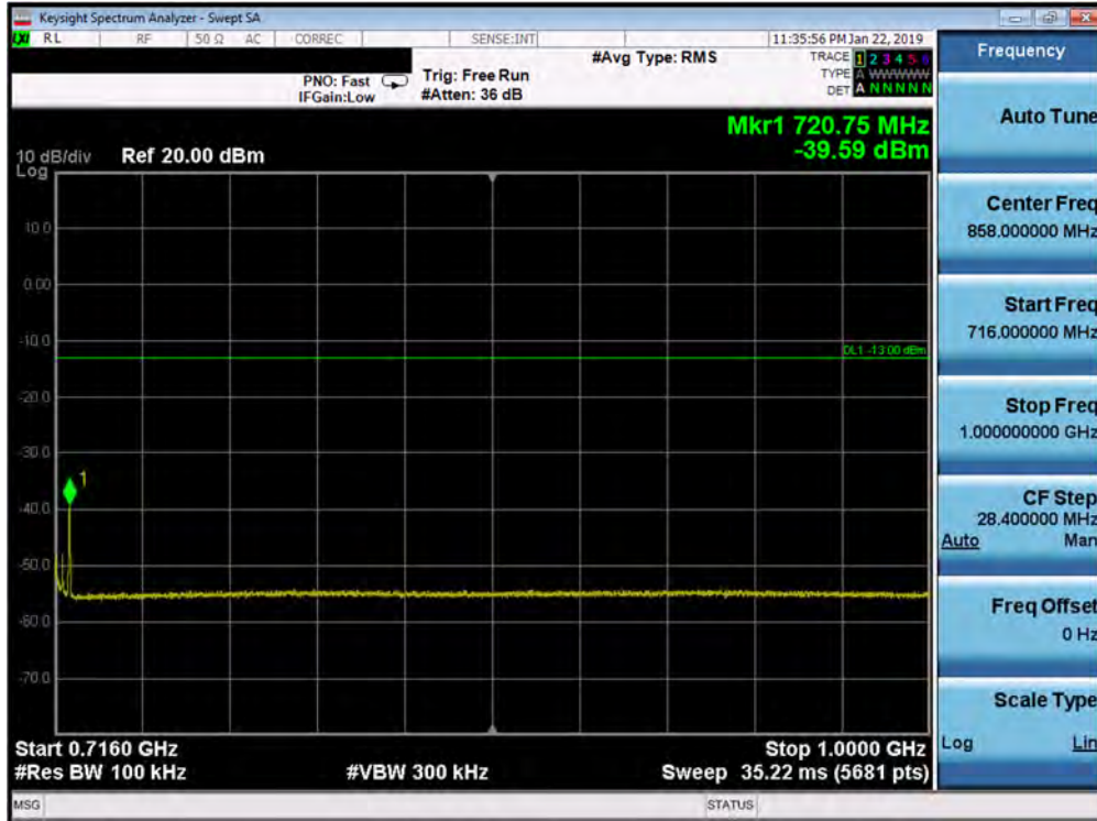
Plot 7-53. Conducted Spurious Plot (Band 12/17 - 10.0MHz QPSK - RB Size 1, RB Offset 0 - Mid Channel)
