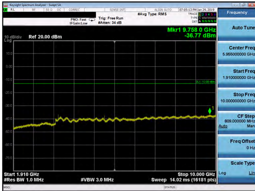
Plot 7-77. Conducted Spurious Plot (Band 2 - 20.0MHz QPSK - RB Size 1, RB Offset 0 - Low Channel)
