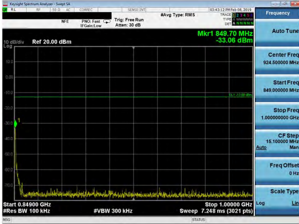
Plot 7-62. Conducted Spurious Plot (Band 5 - 10.0MHz QPSK - RB Size 1, RB Offset 0 - Mid Channel)
