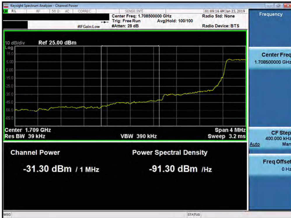
Plot 7-113. Lower Extended Band Edge Plot (Band 66/4 - 1.4MHz QPSK - Full RB Configuration)
