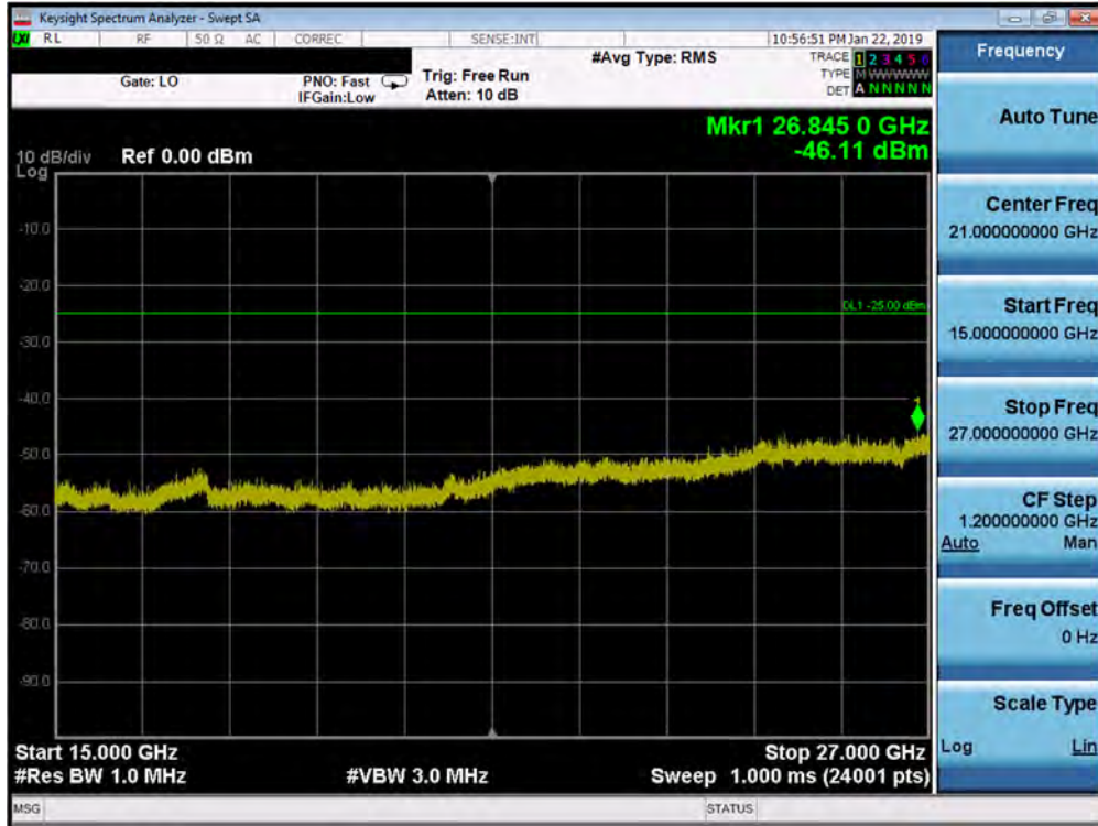
Plot 7-93. Conducted Spurious Plot (Band 41 - 20.0MHz QPSK - RB Size 1, RB Offset 0 - High Channel)
