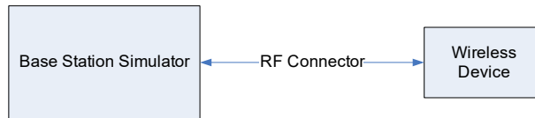
Figure 9-1 Power Measurement Setup
