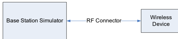
Figure 9-2 Power Measurement Setup
