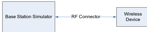
Figure 9-3 Power Measurement Setup
