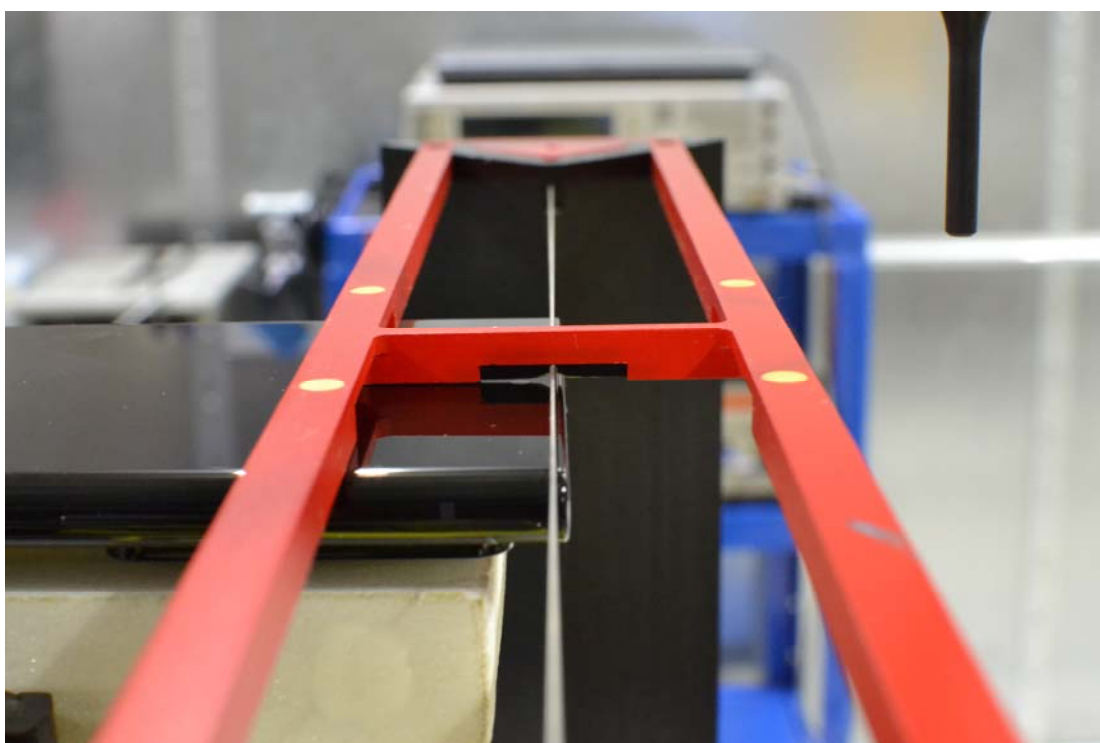
Figure 18-2 HAC Phantom Plane Alignment
