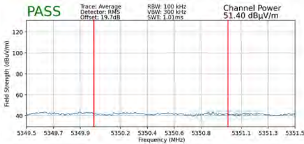
Plot 7-305. Radiated Upper Band Edge Plot SISO ANT2 (Average – UNII Band 2A)
