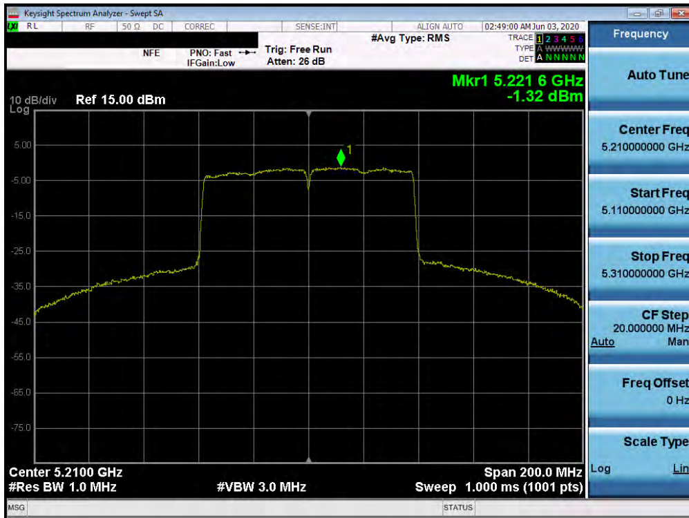
Plot 7-206. Power Spectral Density Plot SISO ANT2 (80MHz BW 802.11ac (UNII Band 1) – Ch. 42)
