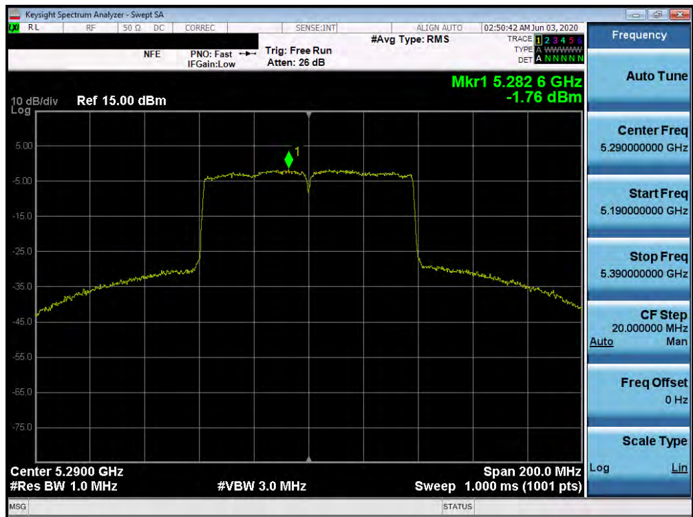
Plot 7-221. Power Spectral Density Plot SISO ANT2 (80MHz BW 802.11ac (UNII Band 2A) – Ch. 58)
