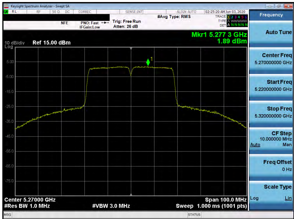
Plot 7-217. Power Spectral Density Plot SISO ANT2 (40MHz BW 802.11n (UNII Band 2A) – Ch. 54)
