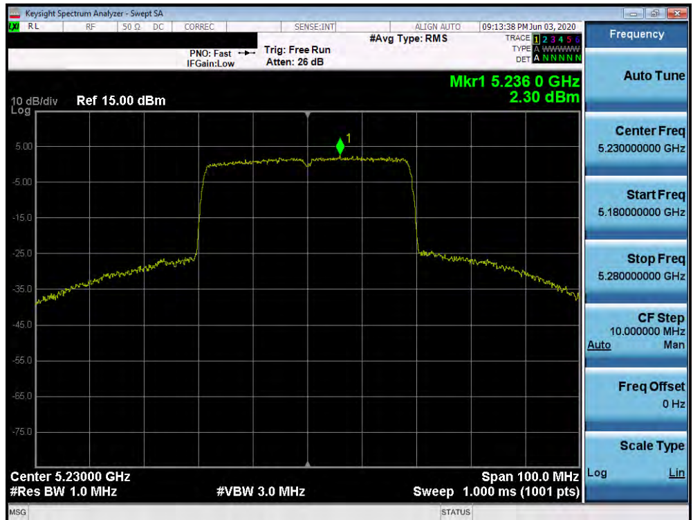
Plot 7-139. Power Spectral Density Plot SISO ANT1 (40MHz BW 802.11ax (UNII Band 1) – Ch. 42)
