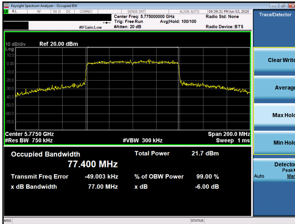
Plot 7-111. 6dB Bandwidth Plot SISO ANT1 (80MHz BW 802.11ax (UNII Band 3) – Ch. 155)
