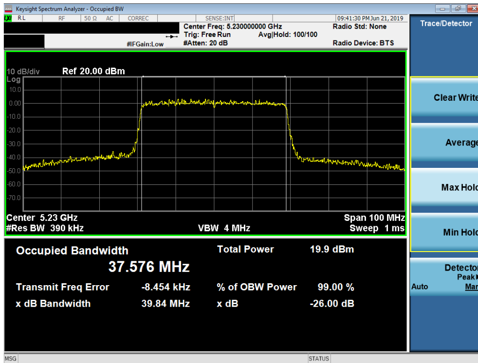
Plot 7-58. 26dB Bandwidth Plot SISO ANT2 (40MHz BW 802.11ax (UNII Band 1) – Ch. 46)
