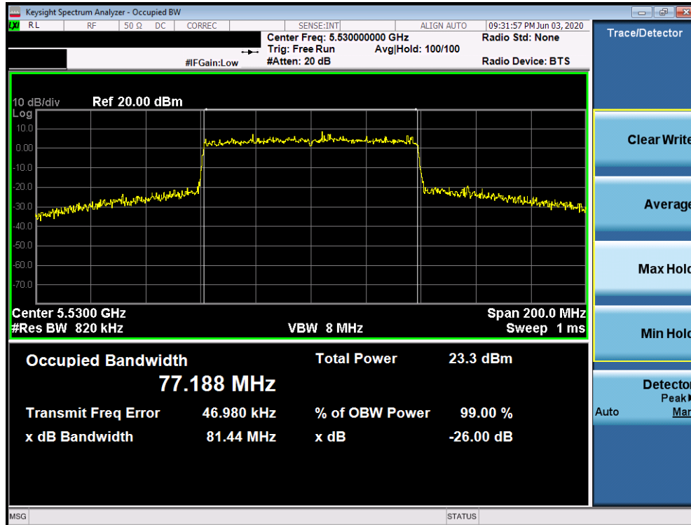
Plot 7-43. 26dB Bandwidth Plot SISO ANT1 (80MHz BW 802.11ax (UNII Band 2C) – Ch. 106)
