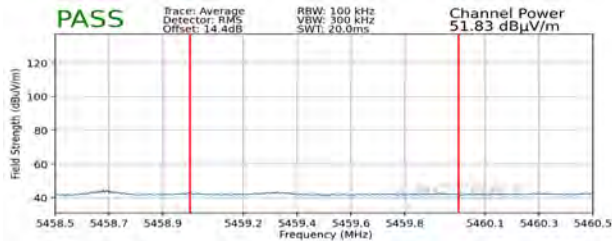
Plot 7-373. Radiated Lower Band Edge Plot SISO ANT1 (Average – UNII Band 2C – 996 Tones)
