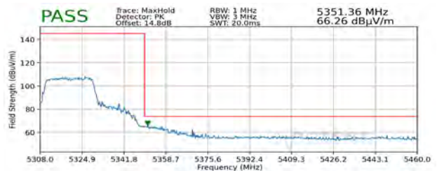
Plot 7-358. Radiated Upper Band Edge Plot SISO ANT1 (Peak – UNII Band 2A – 242 Tones)
