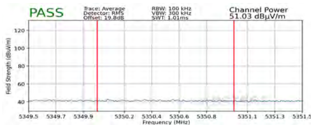
Plot 7-364. Radiated Upper Band Edge Plot SISO ANT1 (Average – UNII Band 2A – 484 Tones)
