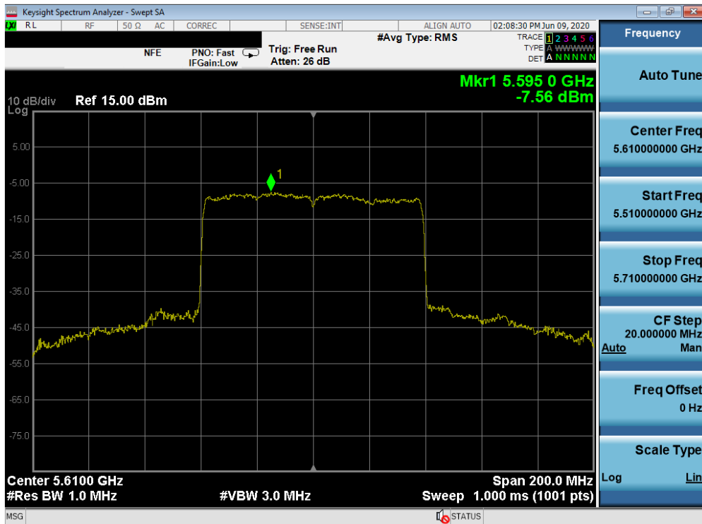
Plot 7-317. Power Spectral Density Plot MIMO ANT2 (80MHz BW 802.11ax – Full Tones (UNII Band 2C) – Ch. 122)
