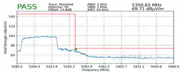
Plot 7-386. Radiated Upper Band Edge Plot SISO ANT2 (Peak – UNII Band 2A – 484 Tones)
