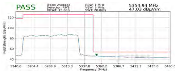
Plot 7-413. Radiated Upper Band Edge Plot MIMO (Average – UNII Band 2A – 996 Tones)
