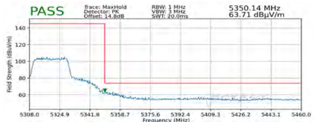
Plot 7-379. Radiated Upper Band Edge Plot SISO ANT2 (Peak – UNII Band 2A – 242 Tones)
