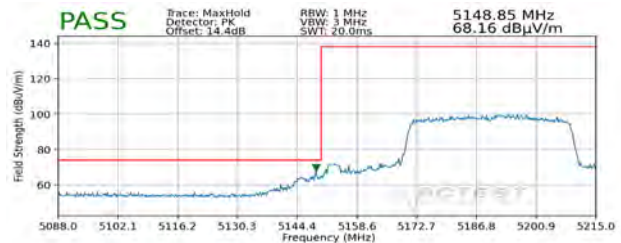
Plot 7-384. Radiated Lower Band Edge Plot SISO ANT2 (Peak – UNII Band 1 – 484 Tones)
