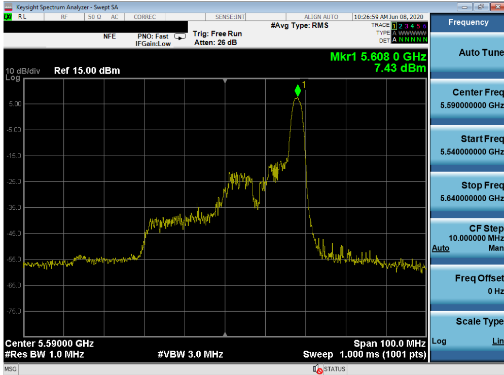
Plot 7-179. Power Spectral Density Plot SISO ANT2 (40MHz BW 802.11ax – 26 Tones (UNII Band 2C) – Ch. 118)
