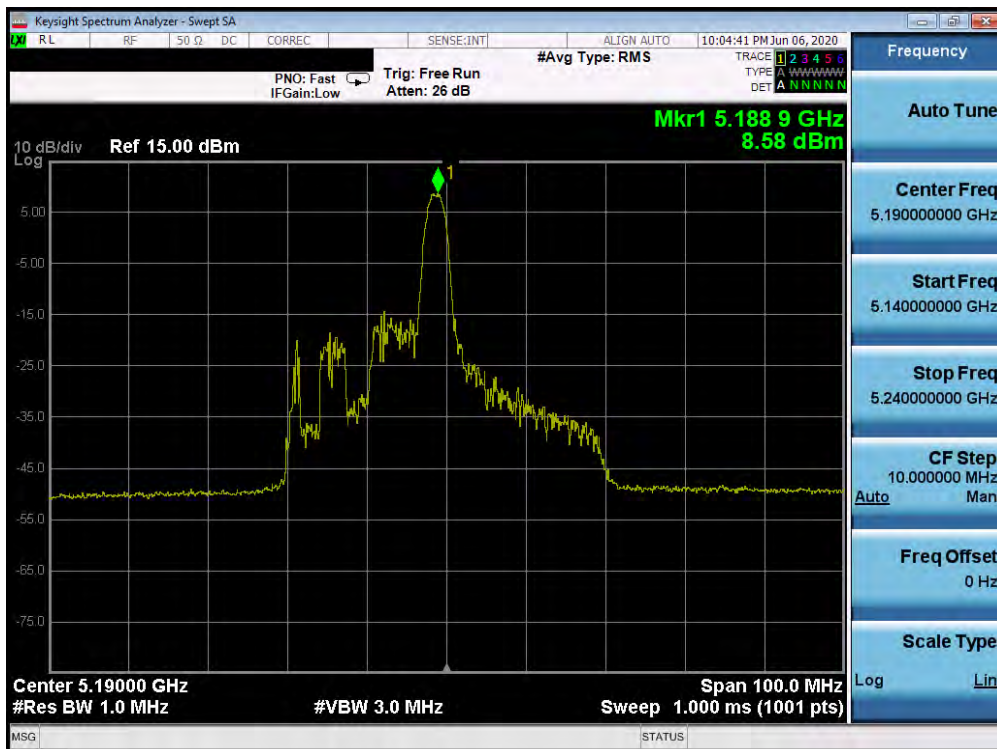
Plot 7-112. Power Spectral Density Plot SISO ANT1 (40MHz BW 802.11ax – 26 Tones (UNII Band 1) – Ch. 38)
