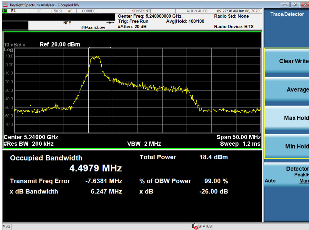
Plot 7-45. 26dB Bandwidth Plot SISO ANT2 (20MHz BW 802.11ax – 26 Tones (UNII Band 1) – Ch. 48)
