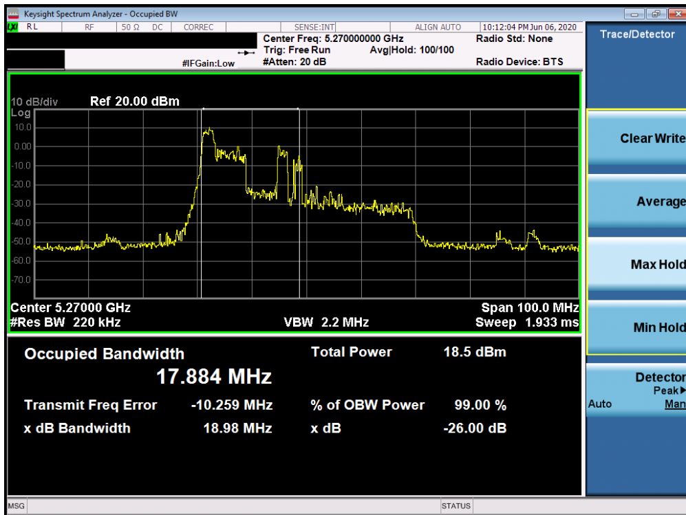
Plot 7-10. 26dB Bandwidth Plot SISO ANT1 (40MHz BW 802.11ax – 26 Tones (UNII Band 2A) – Ch. 54)
