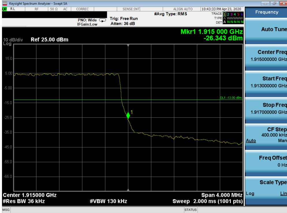
Plot 7-409. Upper Band Edge Plot (Band 25 - 3.0MHz QPSK - Full RB Configuration)
