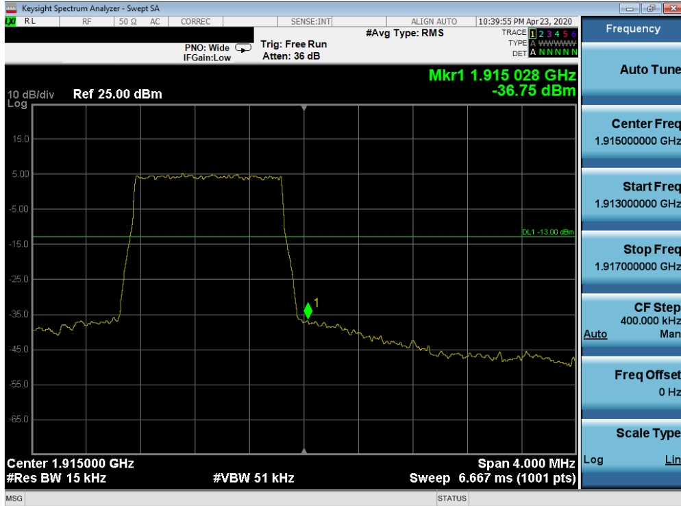
Plot 7-403. Upper Band Edge Plot (Band 25 - 1.4MHz QPSK - Full RB Configuration)
