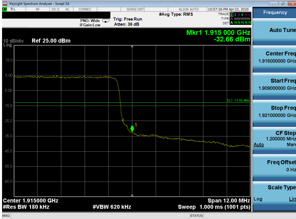
Plot 7-427. Upper Band Edge Plot (Band 25 - 15.0MHz QPSK - Full RB Configuration)
