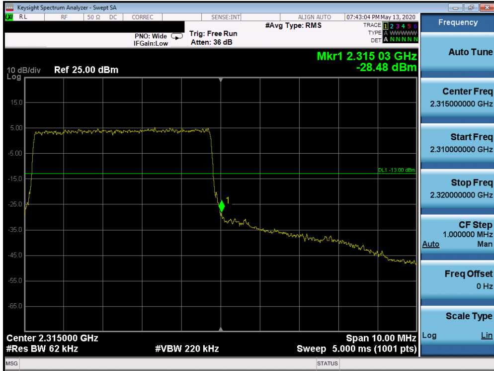
Plot 7-437. Upper Band Edge Plot (Band 30 - 5.0MHz QPSK - Full RB Configuration)
