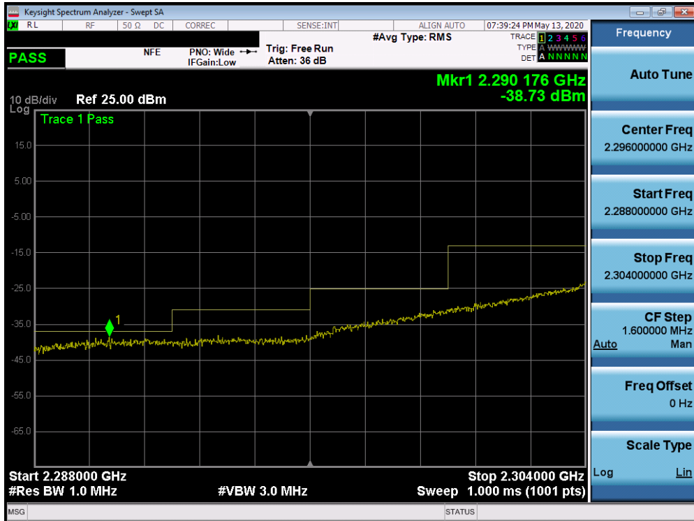
Plot 7-440. Lower Extended Band Edge Plot (Band 30 - 10.0MHz QPSK - Full RB Configuration)
