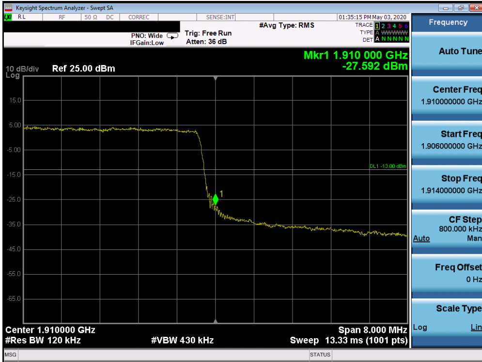
Plot 7-419. Upper Band Edge Plot (Band 2 - 10.0MHz QPSK - Full RB Configuration)
