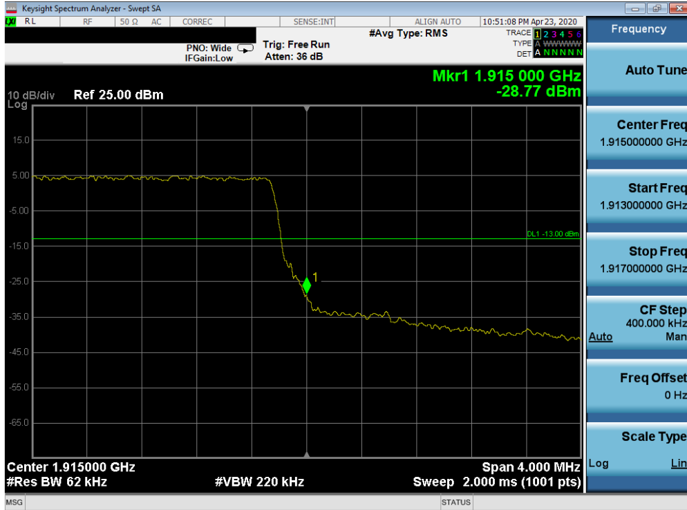
Plot 7-415. Upper Band Edge Plot (Band 25 - 5.0MHz QPSK - Full RB Configuration)
