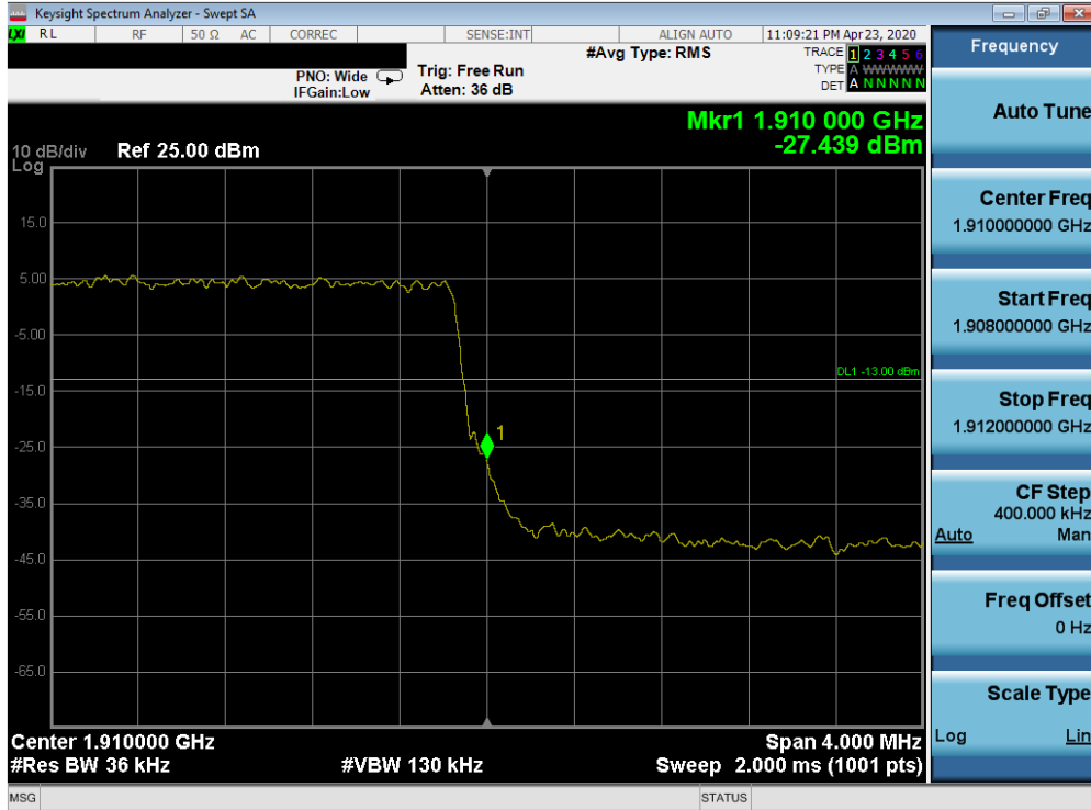
Plot 7-407. Upper Band Edge Plot (Band 2 - 3.0MHz QPSK - Full RB Configuration)
