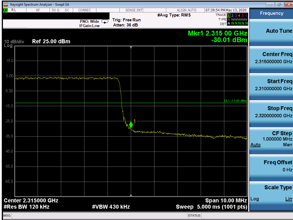
Plot 7-441. Upper Band Edge Plot (Band 30 - 10.0MHz QPSK - Full RB Configuration)
