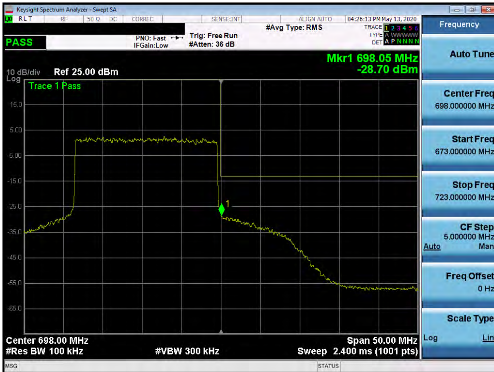
Plot 7-322. Upper Band Edge Plot (n71 - 20MHz DFT-s -OFDM-QPSK - Full RB Configuration)
