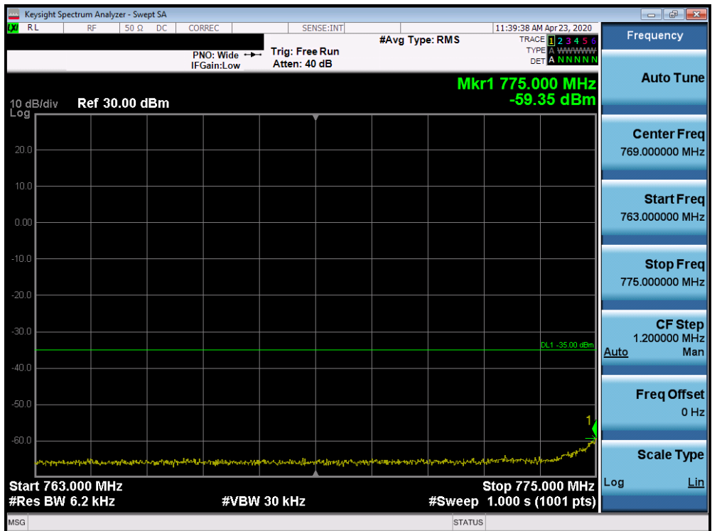
Plot 7-332. Lower Extended Band Edge Plot (Band 13 - 5.0MHz QPSK - Full RB Configuration)
