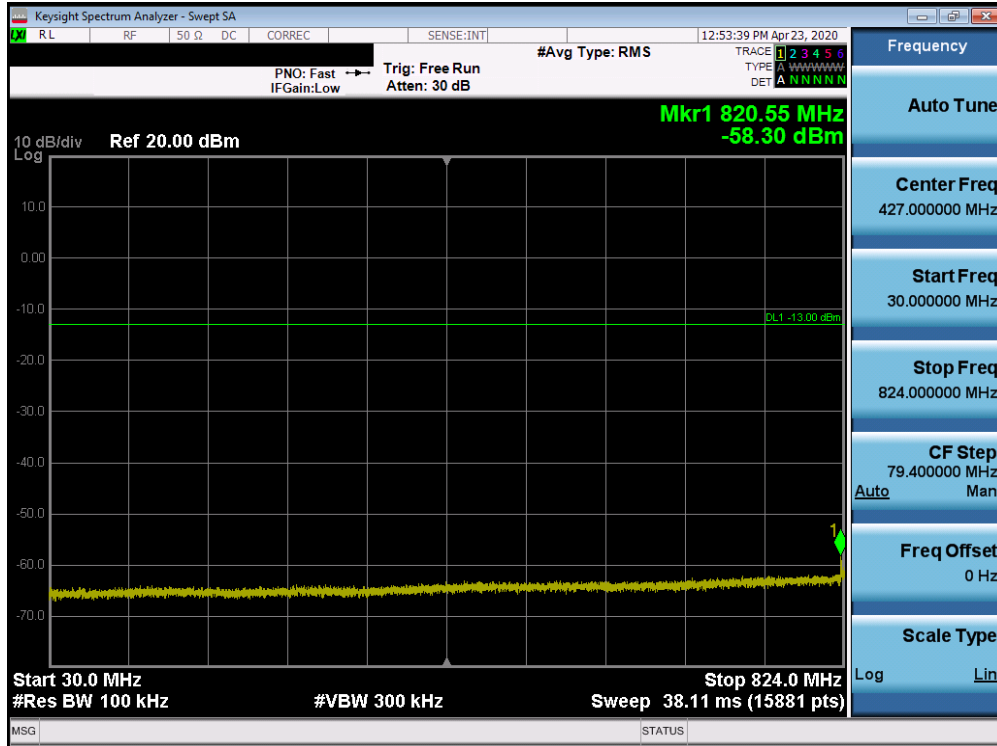
Plot 7-247. Conducted Spurious Plot (Band 5 - 10.0MHz QPSK - RB Size 1, RB Offset 0 - High Channel)
