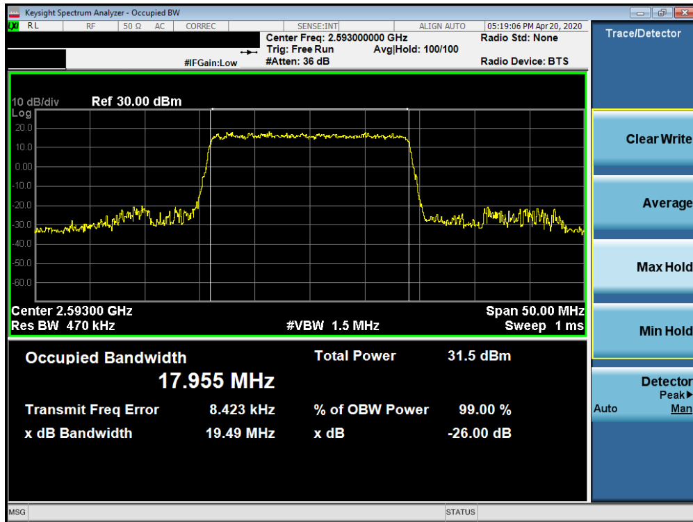
Plot 7-181. Occupied Bandwidth Plot (Band 41 (PC3) - 20.0MHz QPSK - Full RB Configuration)
