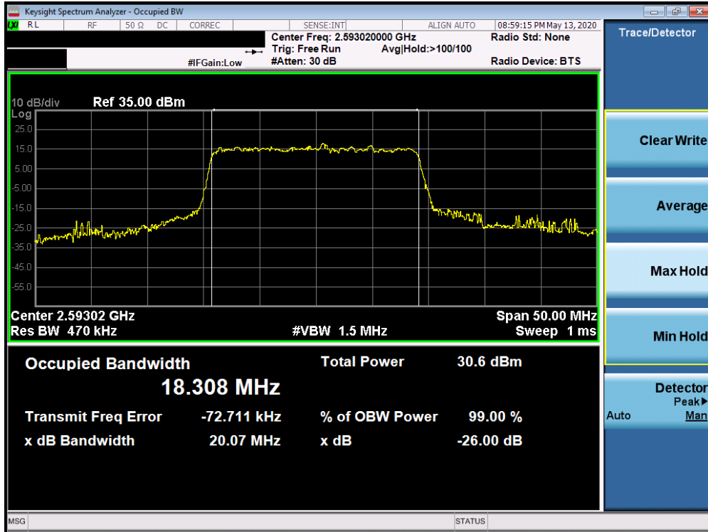
Plot 7-187. Occupied Bandwidth Plot (n41 20MHz 16QAM-CP-OFDM - Full RB Configuration)
