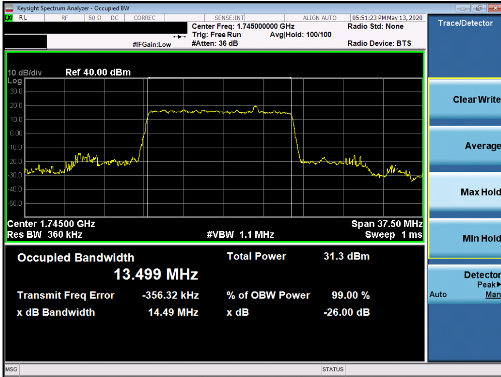
Plot 7-111. Occupied Bandwidth Plot (n66 15MHz BPSK-DFT-s-OFDM - Full RB Configuration)
