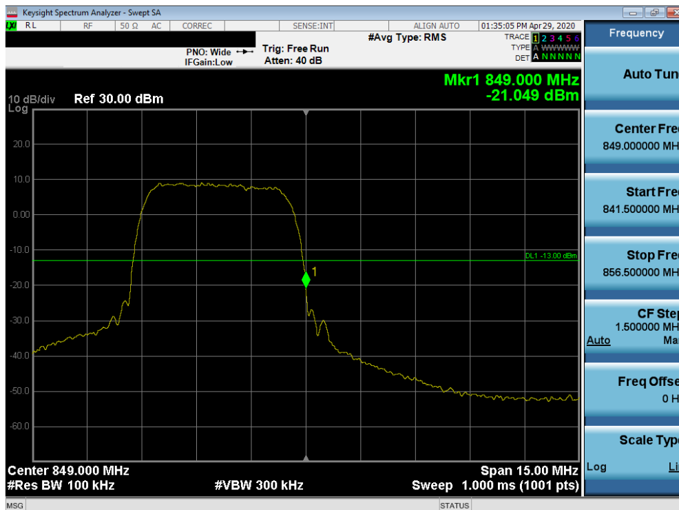
Plot 7-74. Band Edge Plot (Cellular WCDMA Mode - High Channel)
