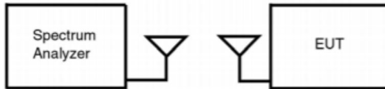
Figure 7-1. Test Instrument and Measurement Setup
