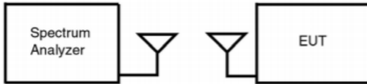
Figure 7-2. Test Instrument and Measurement Setup
