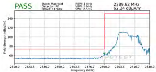
Plot 7-94. Radiated Restricted Lower Band Edge Measurement SISO ANT2 (Peak – 106 Tones)
