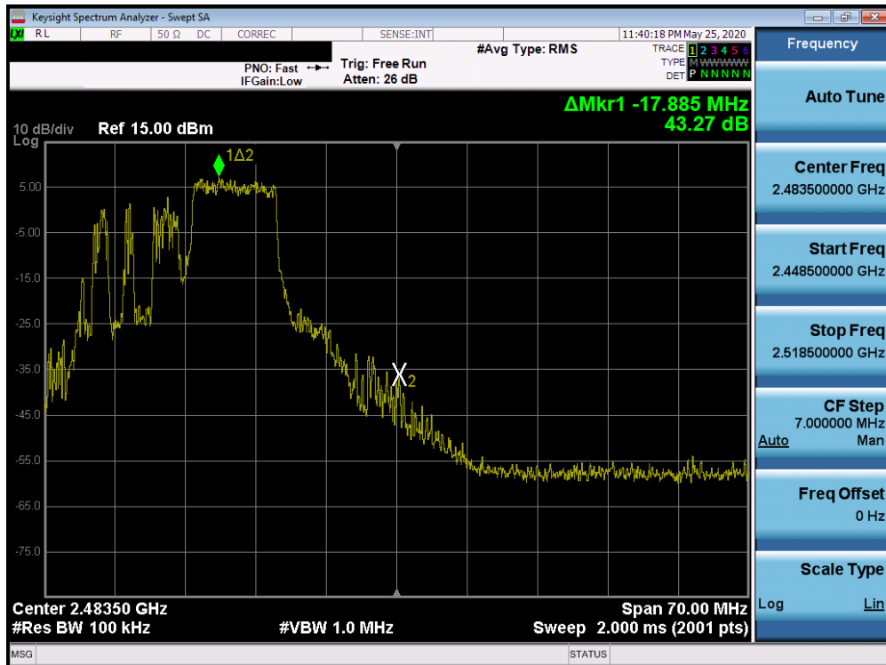
Plot 7-26. Band Edge Plot SISO ANT1 (802.11ax OFDMA – 106 Tones – Ch. 11)
