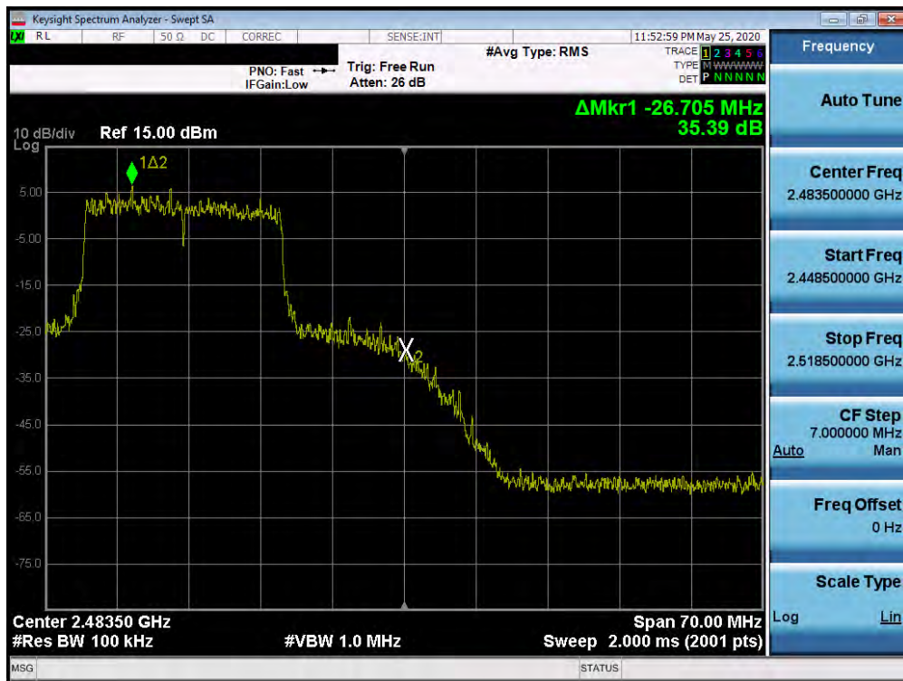
Plot 7-32. Band Edge Plot SISO ANT2 (802.11ax OFDMA – 242 Tones – Ch. 11)
