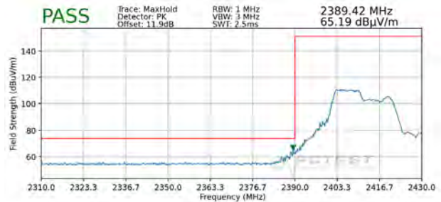
Plot 7-82. Radiated Restricted Lower Band Edge Measurement SISO ANT1 (Peak – 106 Tones)
