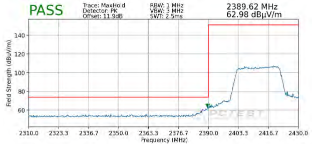
Plot 7-110. Radiated Restricted Lower Band Edge Measurement MIMO (Peak – 242 Tones)
