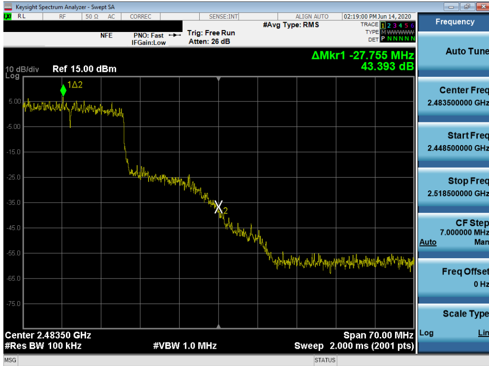
Plot 7-71. Band Edge Plot SISO ANT2 (802.11ax (2.4GHz) – Ch. 10)
