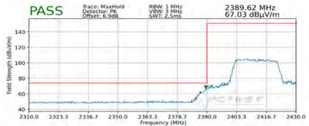
Plot 7-106. Radiated Restricted Lower Band Edge Measurement SISO ANT2 (Peak)
