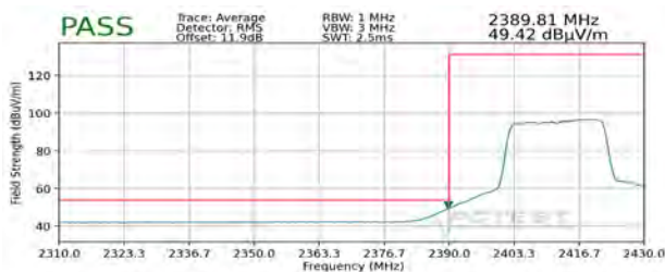
Plot 7-113. Radiated Restricted Lower Band Edge Measurement MIMO (Average)
