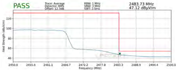
Plot 7-117. Radiated Restricted Lower Band Edge Measurement MIMO (Average)
