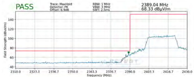
Plot 7-98. Radiated Restricted Lower Band Edge Measurement SISO ANT1 (Peak)
