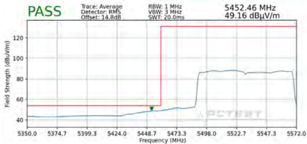
Plot 7-321. Radiated Lower Band Edge Plot SISO ANT2 (Average – UNII Band 2C)
