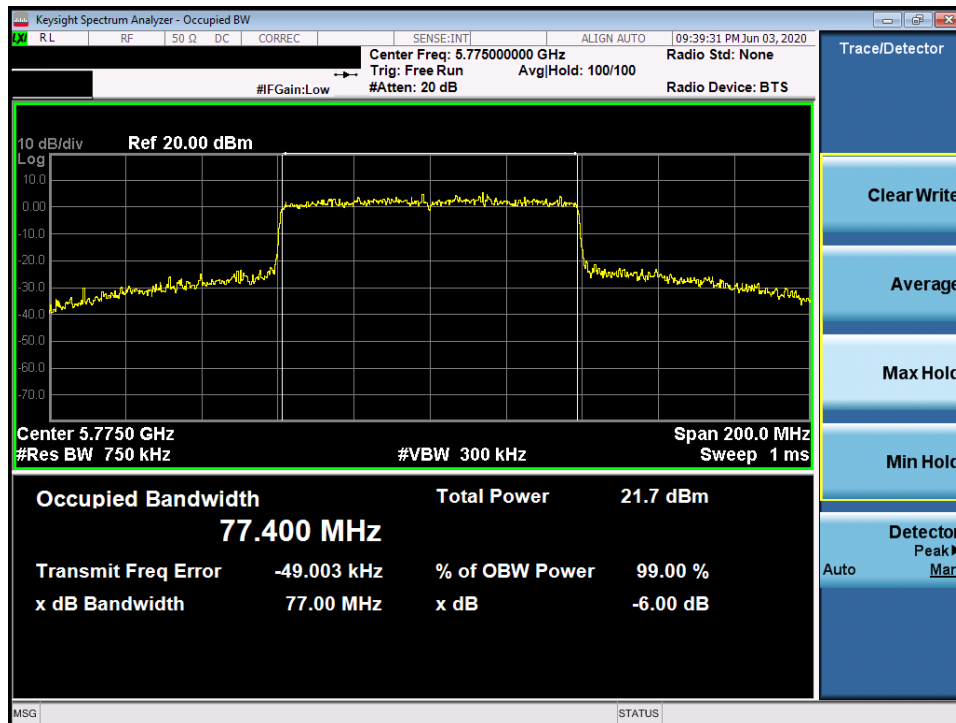
Plot 7-111. 6dB Bandwidth Plot SISO ANT1 (80MHz BW 802.11ax (UNII Band 3) – Ch. 155)
