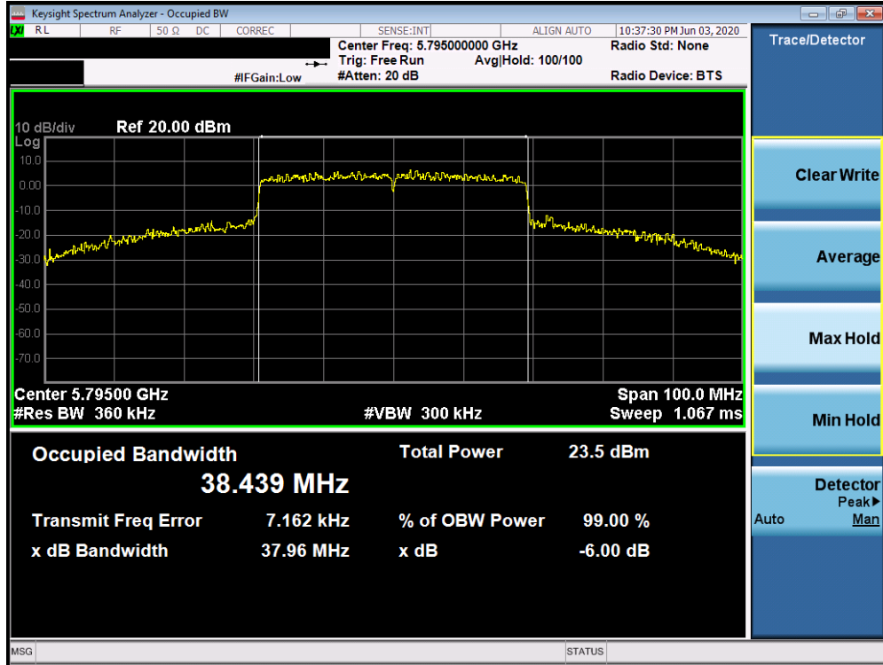
Plot 7-124. 6dB Bandwidth Plot SISO ANT2 (40MHz BW 802.11ax (UNII Band 3) – Ch. 159)
