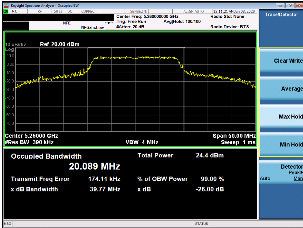
Plot 7-16. 26dB Bandwidth Plot SISO ANT1 (20MHz BW 802.11n (UNII Band 2A) – Ch. 52)
