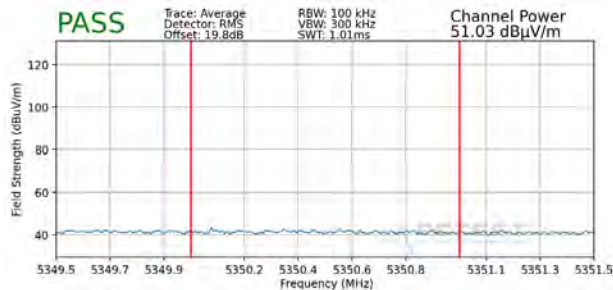
Plot 7-364. Radiated Upper Band Edge Plot SISO ANT1 (Average – UNII Band 2A – 484 Tones)
