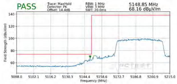
Plot 7-384. Radiated Lower Band Edge Plot SISO ANT2 (Peak – UNII Band 1 – 484 Tones)
