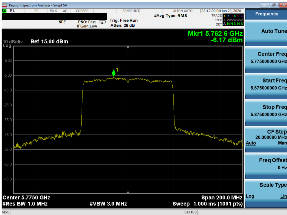
Plot 7-324. Power Spectral Density Plot MIMO ANT2 (80MHz BW 802.11ax – Full Tones (UNII Band 3) – Ch. 155)
