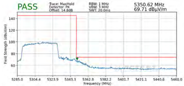
Plot 7-386. Radiated Upper Band Edge Plot SISO ANT2 (Peak – UNII Band 2A – 484 Tones)
