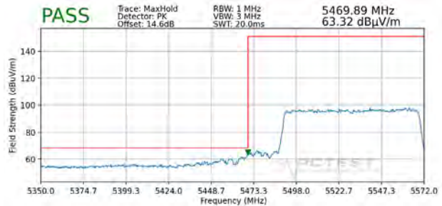
Plot 7-416. Radiated Lower Band Edge Plot MIMO (Peak – UNII Band 2C – 996 Tones)
