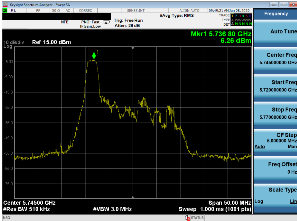
Plot 7-184. Power Spectral Density Plot SISO ANT2 (20MHz BW 802.11ax – 26 Tones (UNII Band 3) – Ch. 149)
