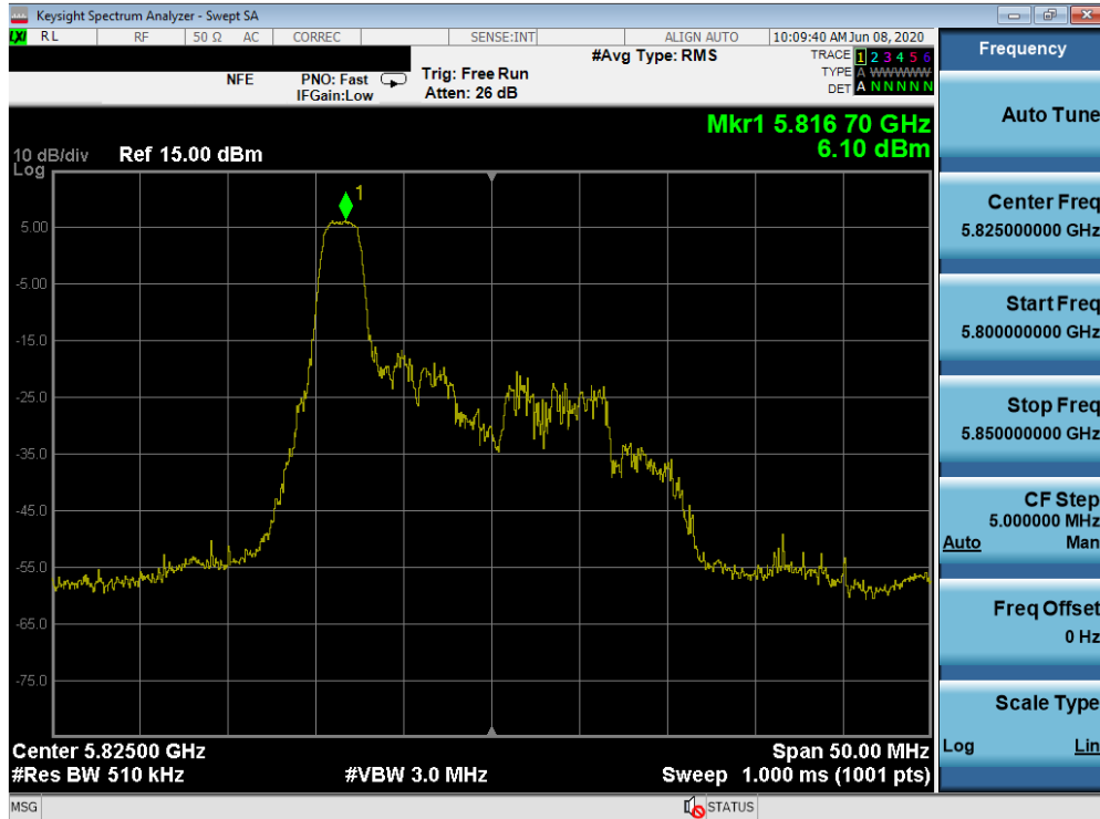
Plot 7-186. Power Spectral Density Plot SISO ANT2 (20 MHz BW 802.11ax – 26 Tones (UNII Band 3) – Ch. 165)
