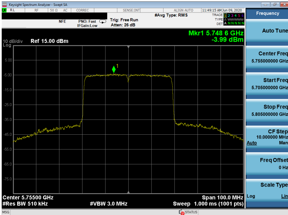
Plot 7-268. Power Spectral Density Plot MIMO ANT1 (40MHz BW 802.11ax – Full Tones (UNII Band 3) – Ch. 151)
