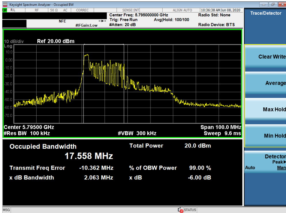
Plot 7-101. 6dB Bandwidth Plot SISO ANT2 (40MHz BW 802.11ax – 26 Tones (UNII Band 3) – Ch. 159)
