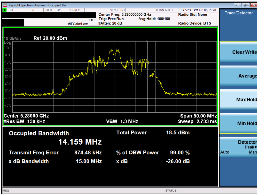
Plot 7-8. 26dB Bandwidth Plot SISO ANT1 (20MHz BW 802.11ax – 26 Tones (UNII Band 2A) – Ch. 56)
