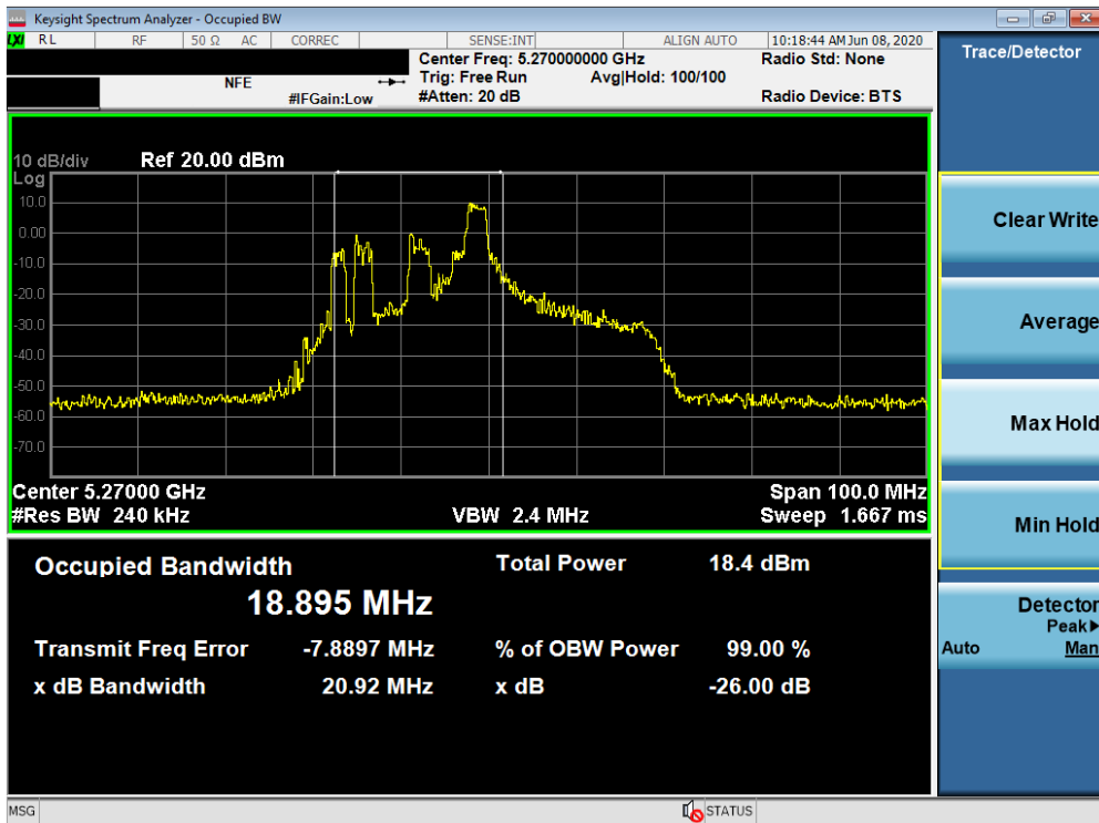
Plot 7-52. 26dB Bandwidth Plot SISO ANT2 (40MHz BW 802.11ax – 26 Tones (UNII Band 2A) – Ch. 54)
