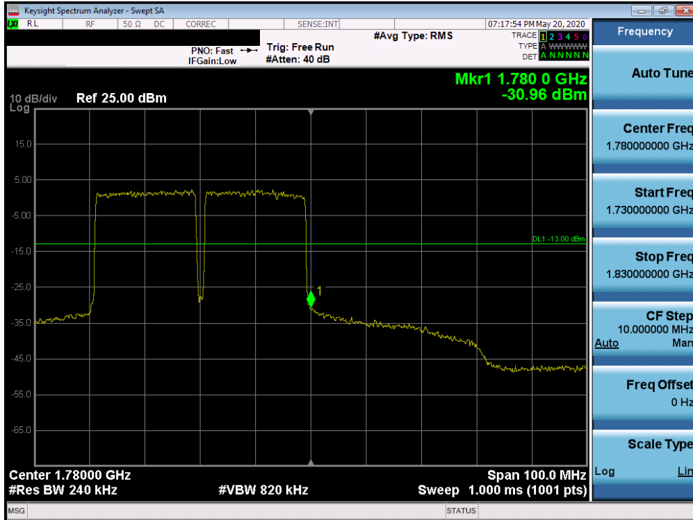
Plot 7-715. Upper Band Edge Plot (Band 66 QPSK – PCC:20 MHz SCC:20 MHz – Full RB)
