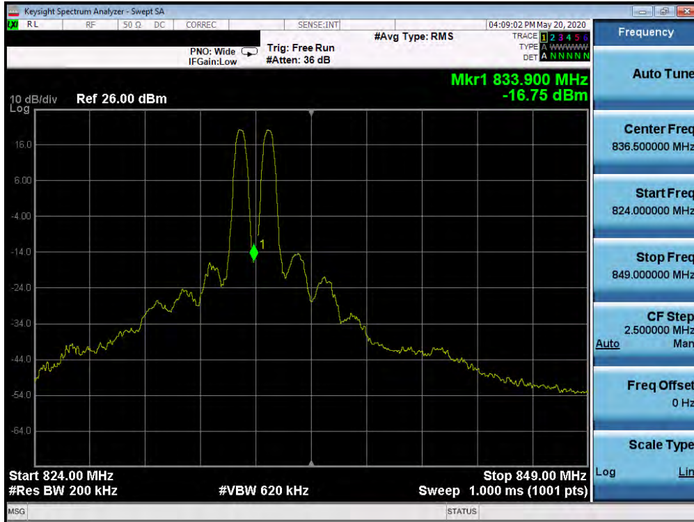
Plot 7-692. Conducted Spurious Plot (Band 5 – 10.0MHz QPSK – PCC 1/49 SCC 1/0 – Low Channel)
