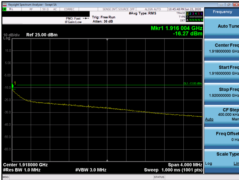
Plot 7-551. Upper Extended Band Edge Plot (n25 - 5MHz DFT-s-OFDM-QPSK - Full RB Configuration)
