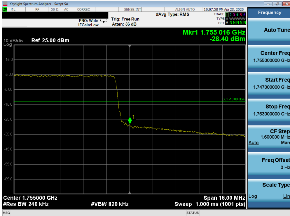
Plot 7-490. Upper Band Edge Plot (Band 4 - 20.0MHz QPSK - Full RB Configuration)
