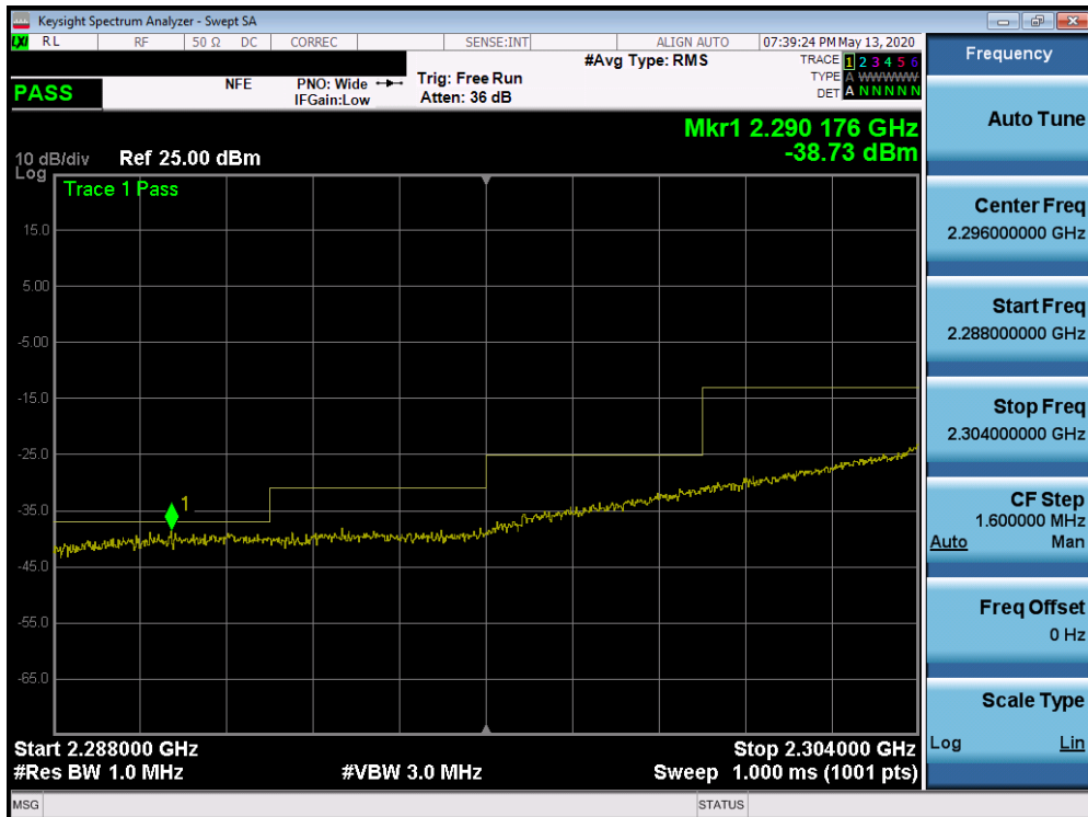
Plot 7-575. Lower Extended Band Edge Plot (Band 30 - 10.0MHz QPSK - Full RB Configuration)
