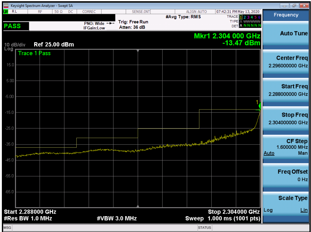
Plot 7-571. Lower Extended Band Edge Plot (Band 30 - 5.0MHz QPSK - Full RB Configuration)
