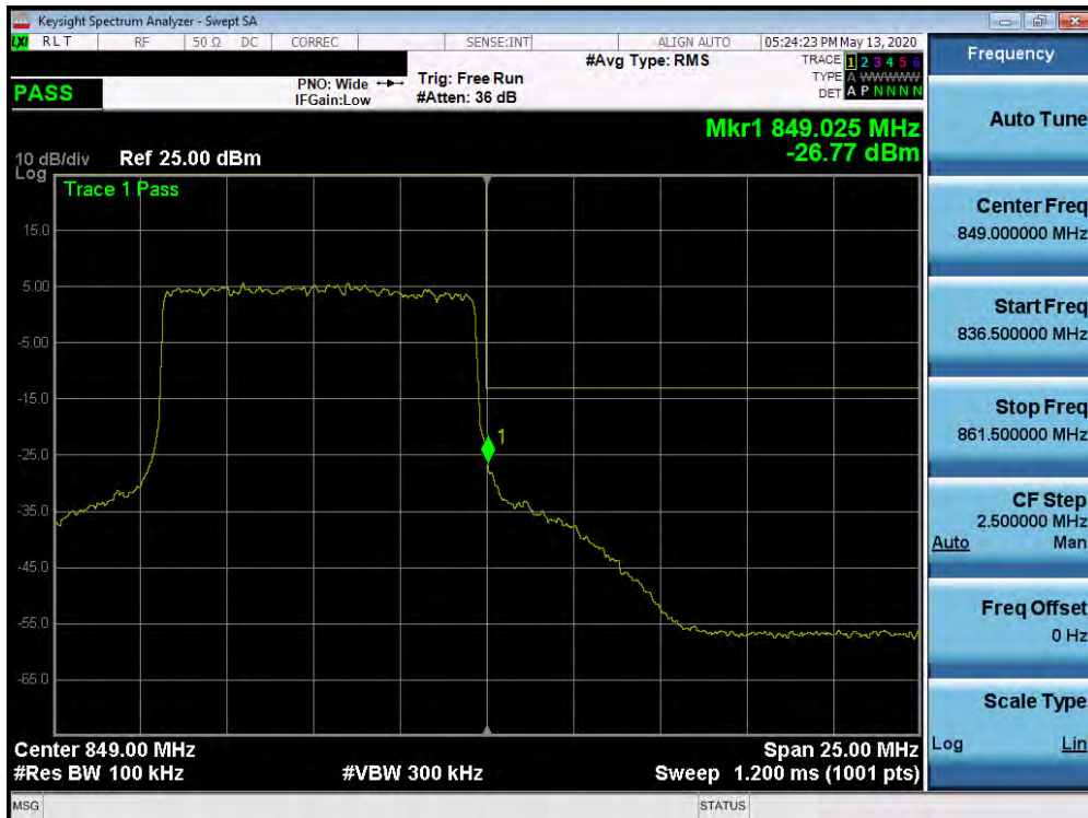
Plot 7-453. Upper Band Edge Plot (n5 – 10.0MHz DFT-s-OFDM BPSK - Full RB Configuration)
