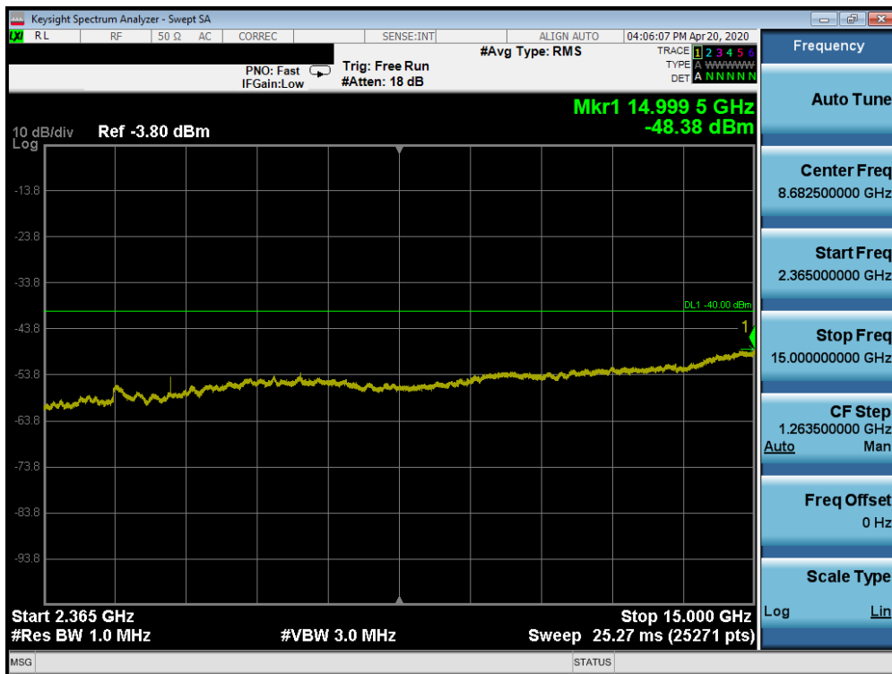
Plot 7-372. Conducted Spurious Plot (Band 30 - 10.0MHz QPSK - RB Size 1, RB Offset 0 - Mid Channel)
