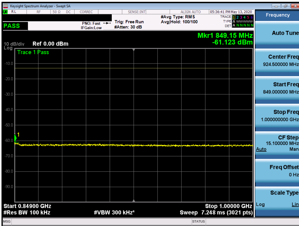
Plot 7-334. Conducted Spurious Plot (n5 - 20.0MHz DFT-s-OFDM BPSK - RB Size 1, RB Offset 0 - High Channel)
