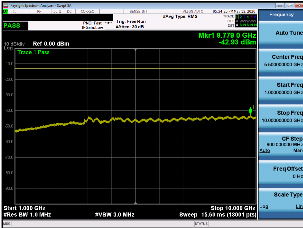
Plot 7-329. Conducted Spurious Plot (n5 - 20.0MHz DFT-s-OFDM BPSK - RB Size 1, RB Offset 0 - Low Channel)
