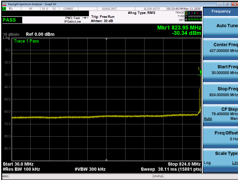
Plot 7-327. Conducted Spurious Plot (n5 - 20.0MHz DFT-s-OFDM BPSK - RB Size 1, RB Offset 0 - Low Channel)
