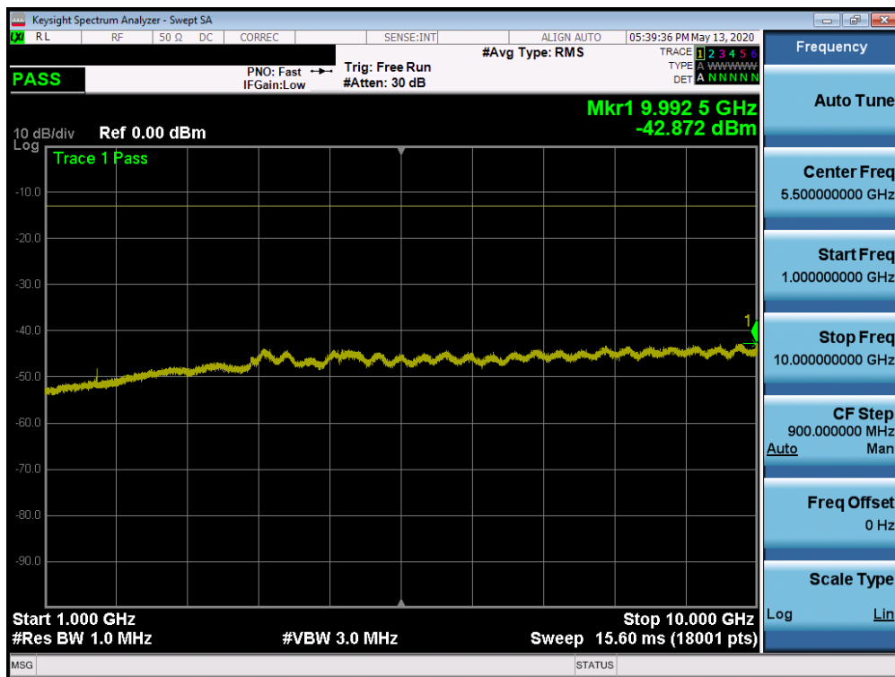
Plot 7-332. Conducted Spurious Plot (n5 - 20.0MHz DFT-s-OFDM BPSK - RB Size 1, RB Offset 0 - Mid Channel)
