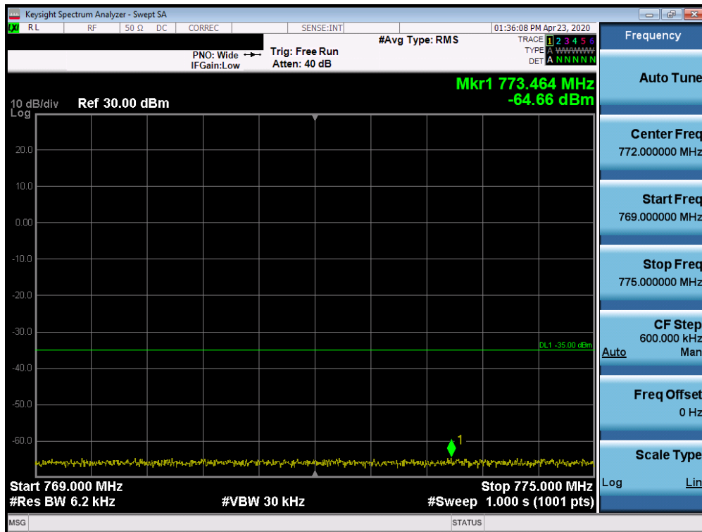
Plot 7-56. Lower Extended Band Edge Plot (Band 14 - 5MHz QPSK - Full RB Configuration)
