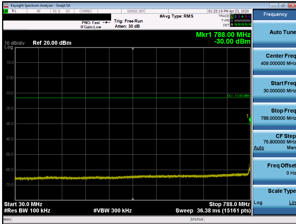
Plot 7-40. Conducted Spurious Plot (LTE Band 14 - 10MHz QPSK - RB Size 1, RB Offset 0)
