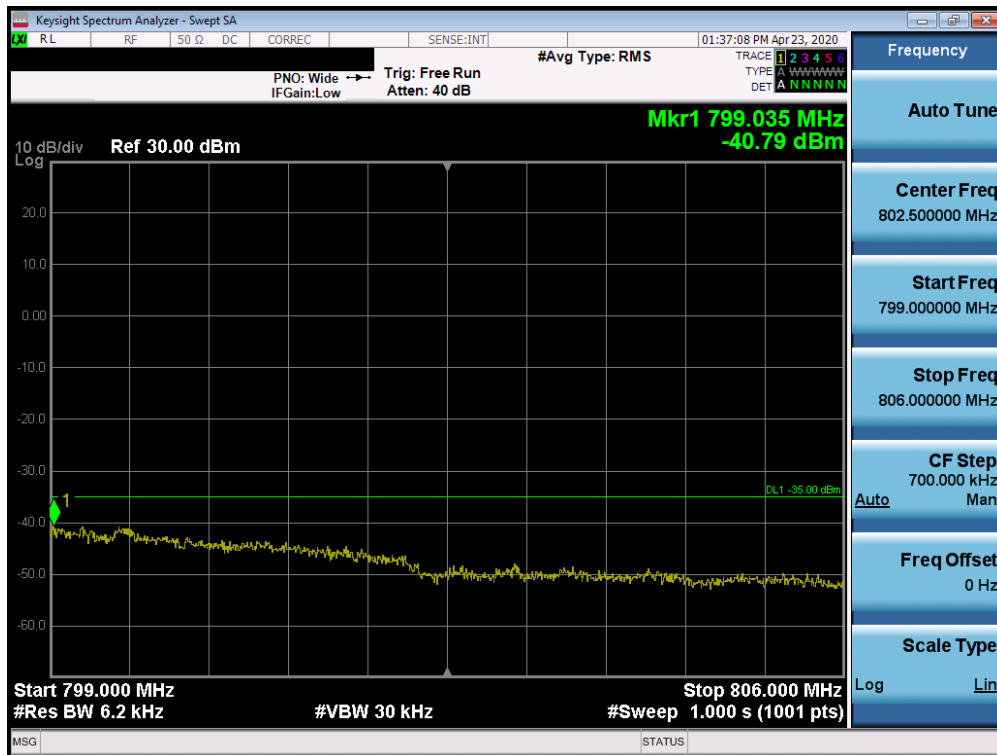
Plot 7-58. Upper Extended Band Edge Plot (Band 14 - 5MHz QPSK - Full RB Configuration)
