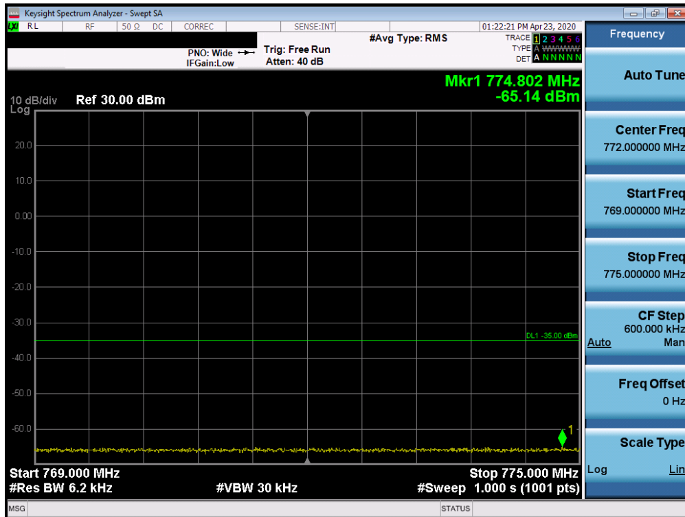
Plot 7-52. Lower Extended Band Edge Plot (Band 14 - 10MHz QPSK - Full RB Configuration)
