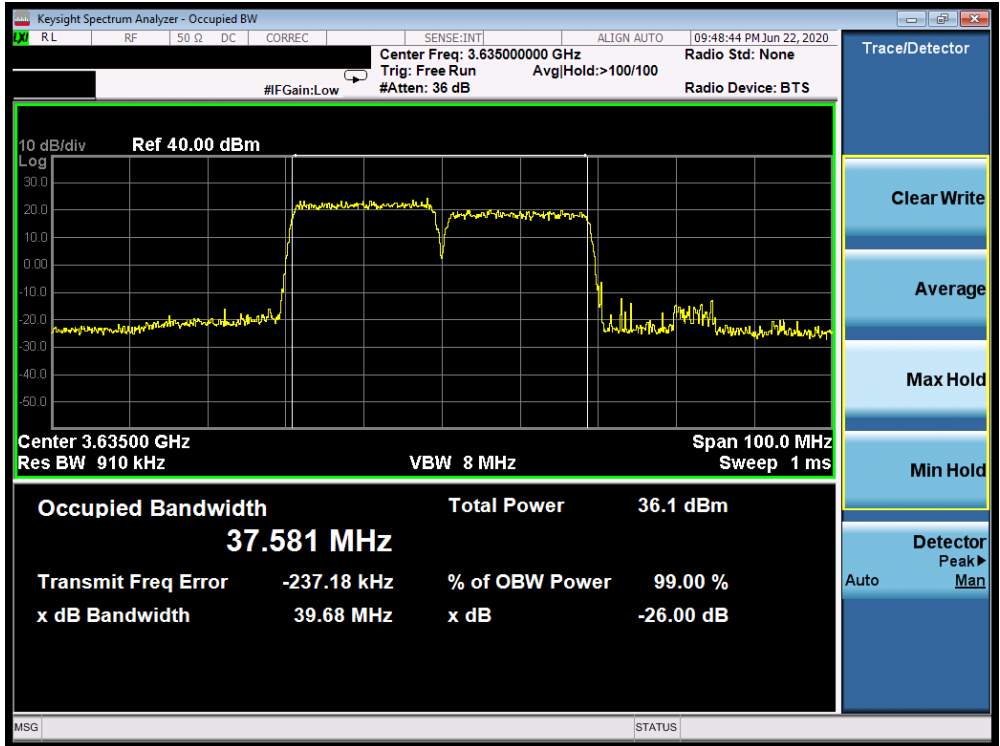
Plot 7-29. Occupied Bandwidth Plot (LTE Band 48 - 40.0MHz QPSK - Full RB Configuration)
