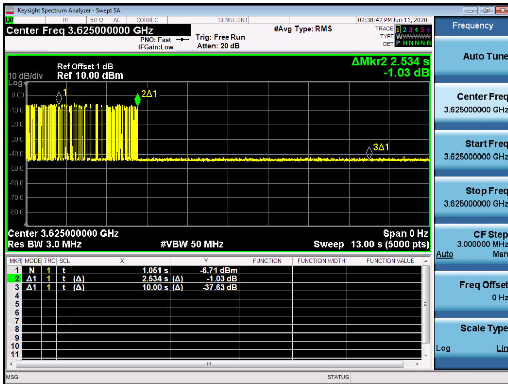
Plot 7-77. Run#1 End User Device Discontinues Operations within 10s
