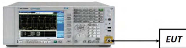
Figure 7-3. Test Instrument & Measurement Setup
