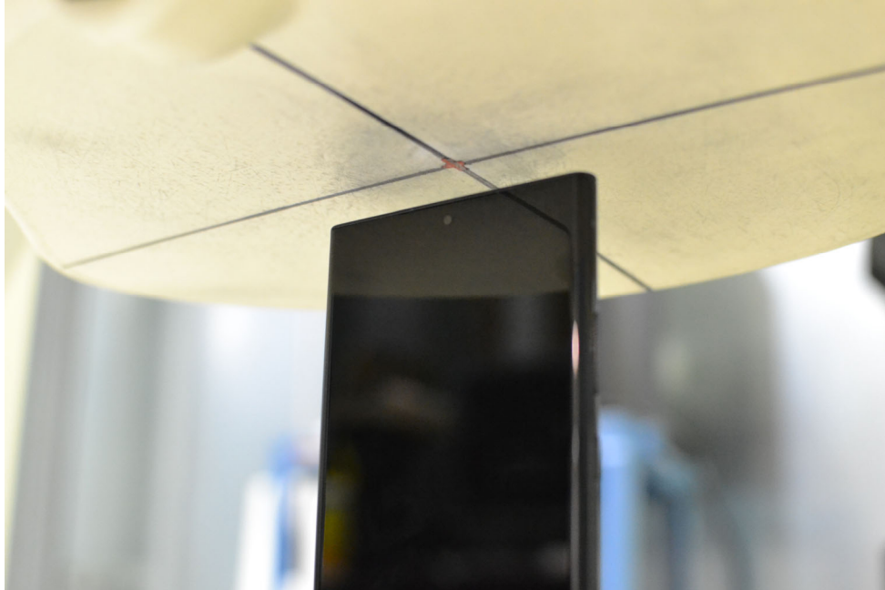
SAR Test Setup Photo 11 – Top Side at 10 mm
