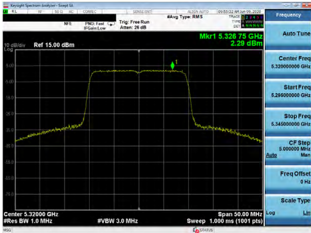
Plot 7-306. Power Spectral Density Plot MIMO ANT2 (20MHz BW 802.11ax – Full Tones (UNII Band 2A) – Ch. 64)
