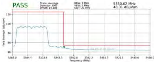
Plot 7-406. Radiated Upper Band Edge Plot MIMO (Average – UNII Band 2A – 484 Tones)
