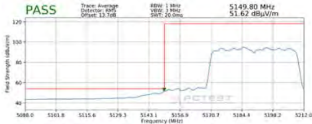
Plot 7-404. Radiated Lower Band Edge Plot MIMO (Average – UNII Band 1 – 484 Tones)
