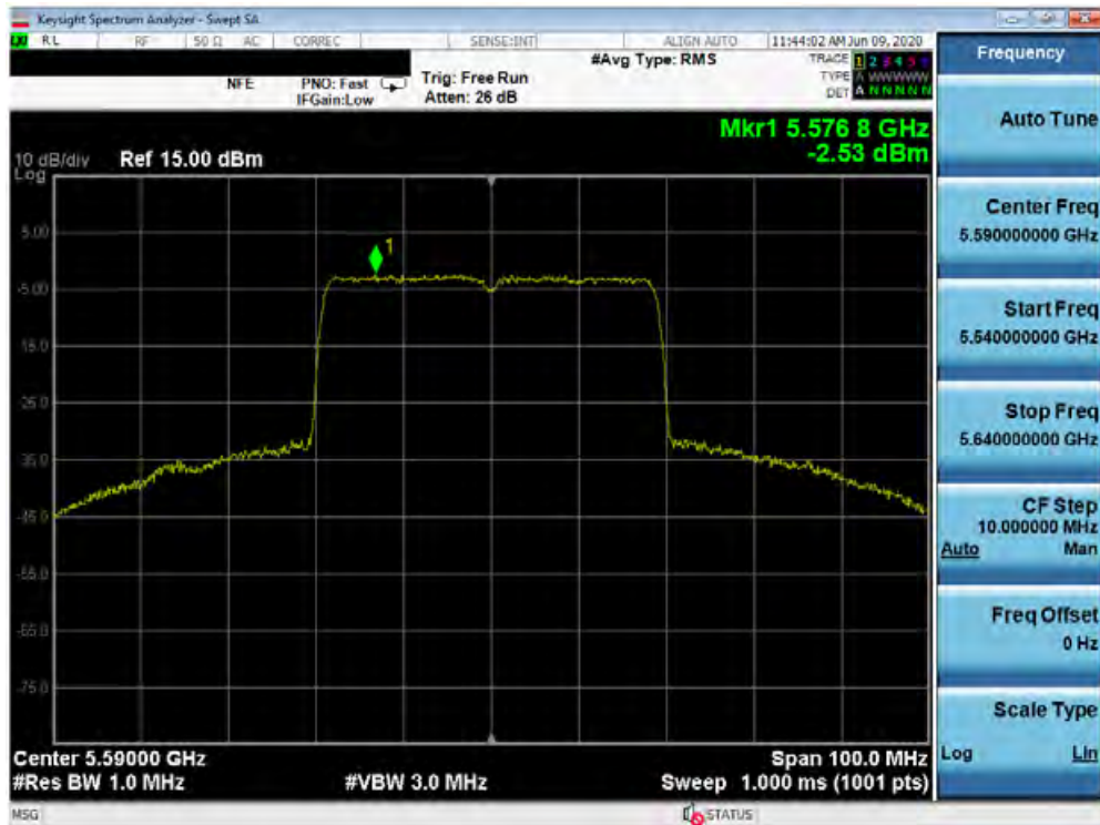
Plot 7-314. Power Spectral Density Plot MIMO ANT2 (40MHz BW 802.11ax – Full Tones (UNII Band 2C) – Ch. 118)
