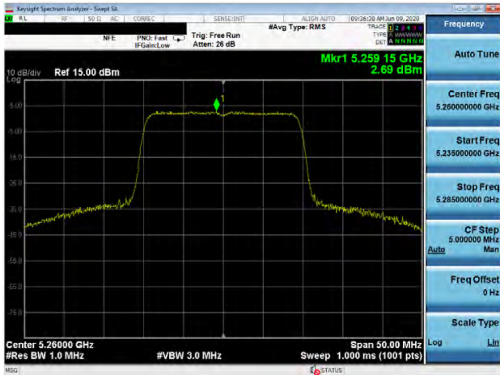
Plot 7-304. Power Spectral Density Plot MIMO ANT2 (20MHz BW 802.11ax – Full Tones (UNII Band 2A) – Ch. 52)
