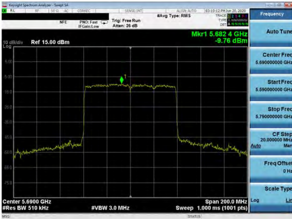
Plot 7-318. Power Spectral Density Plot MIMO ANT2 (80MHz BW 802.11ax – Full Tones (UNII Band 2C) – Ch. 138)
