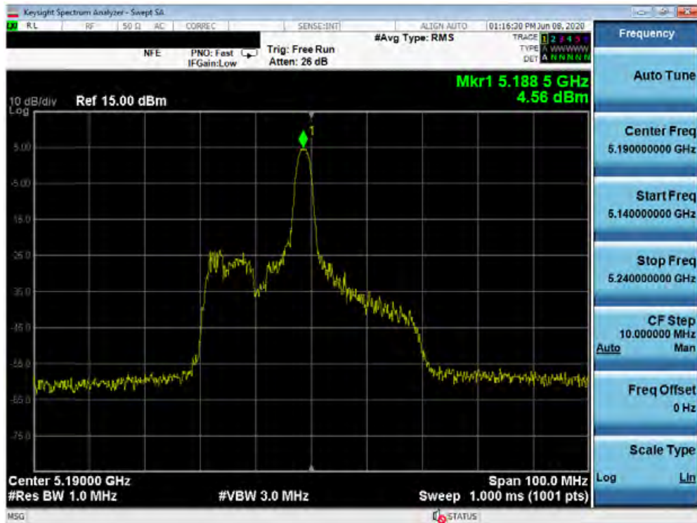
Plot 7-220. Power Spectral Density Plot MIMO ANT1 (40MHz BW 802.11ax – 26 Tones (UNII Band 1) – Ch. 38)
