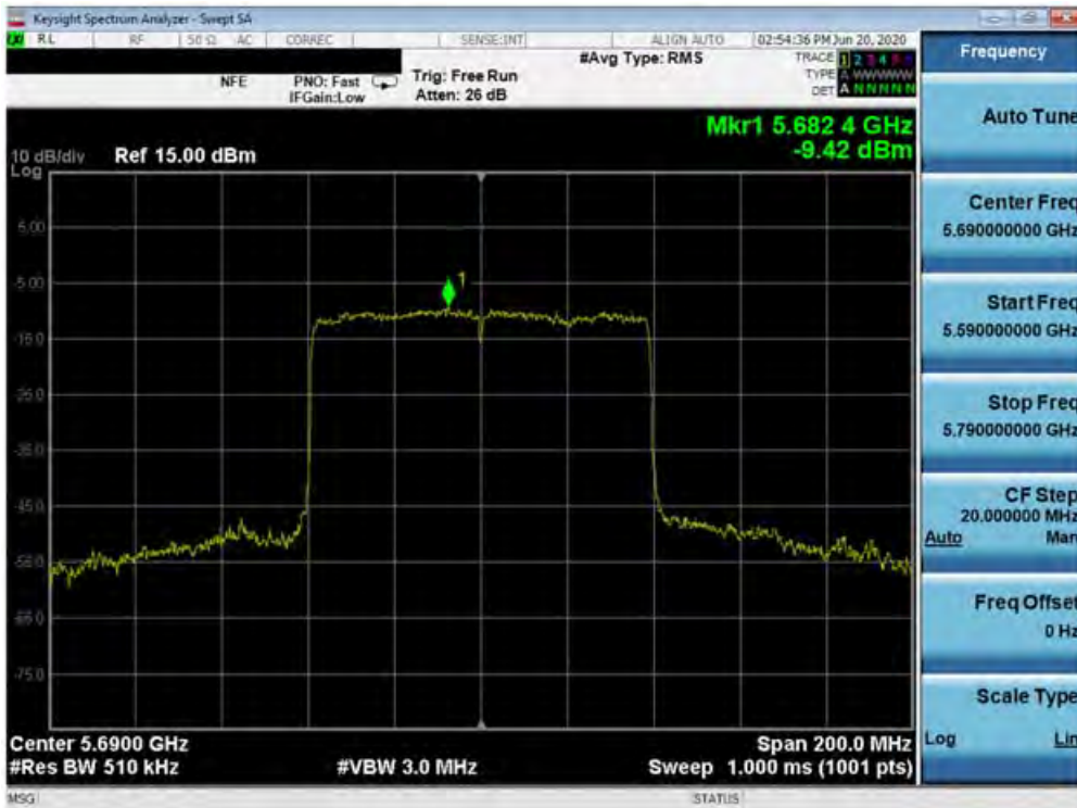
Plot 7-264. Power Spectral Density Plot MIMO ANT1 (80MHz BW 802.11ax – Full Tones (UNII Band 2C) – Ch. 138)
