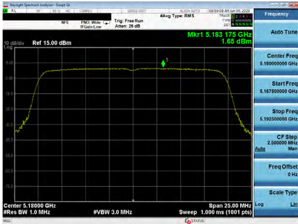
Plot 7-244. Power Spectral Density Plot MIMO ANT1 (20MHz BW 802.11ax – Full Tones (UNII Band 1) – Ch. 36)
