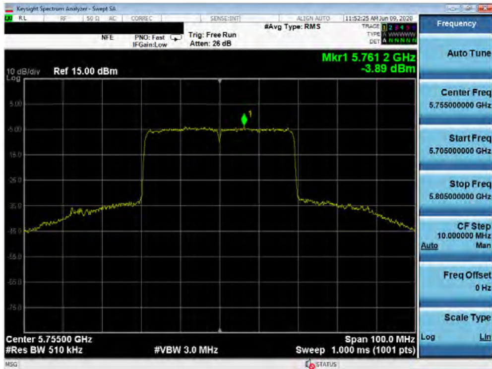
Plot 7-322. Power Spectral Density Plot MIMO ANT2 (40MHz BW 802.11ax – Full Tones (UNII Band 3) – Ch. 151)
