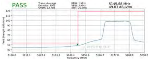
Plot 7-397. Radiated Lower Band Edge Plot MIMO (Average – UNII Band 1 – 242 Tones)
