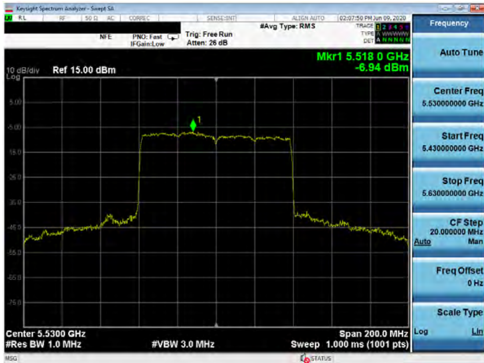
Plot 7-316. Power Spectral Density Plot MIMO ANT2 (80MHz BW 802.11ax – Full Tones (UNII Band 2C) – Ch. 106)
