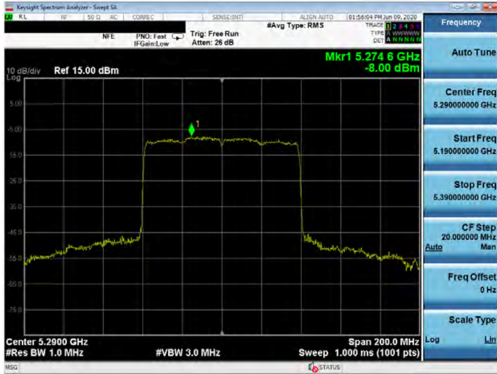
Plot 7-309. Power Spectral Density Plot MIMO ANT2 (80MHz BW 802.11ax – Full Tones (UNII Band 2A) – Ch. 58)
