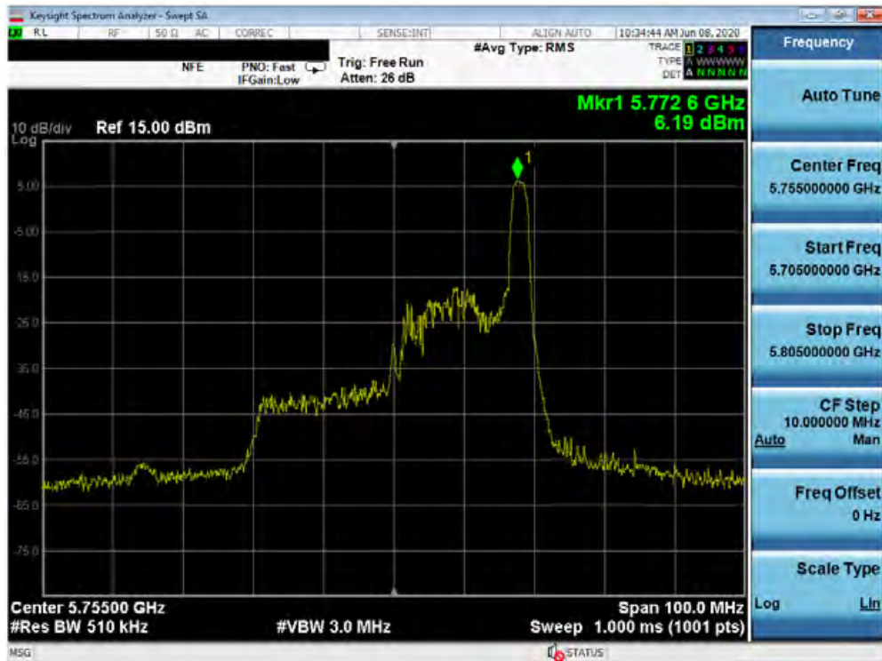
Plot 7-187. Power Spectral Density Plot SISO ANT2 (40MHz BW 802.11ax – 26 Tones (UNII Band 3) – Ch. 151)
