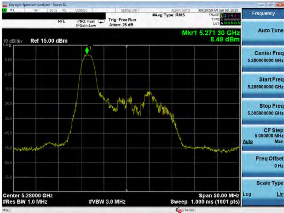
Plot 7-170. Power Spectral Density Plot SISO ANT2 (20MHz BW 802.11ax – 26 Tones (UNII Band 2A) – Ch. 56)
