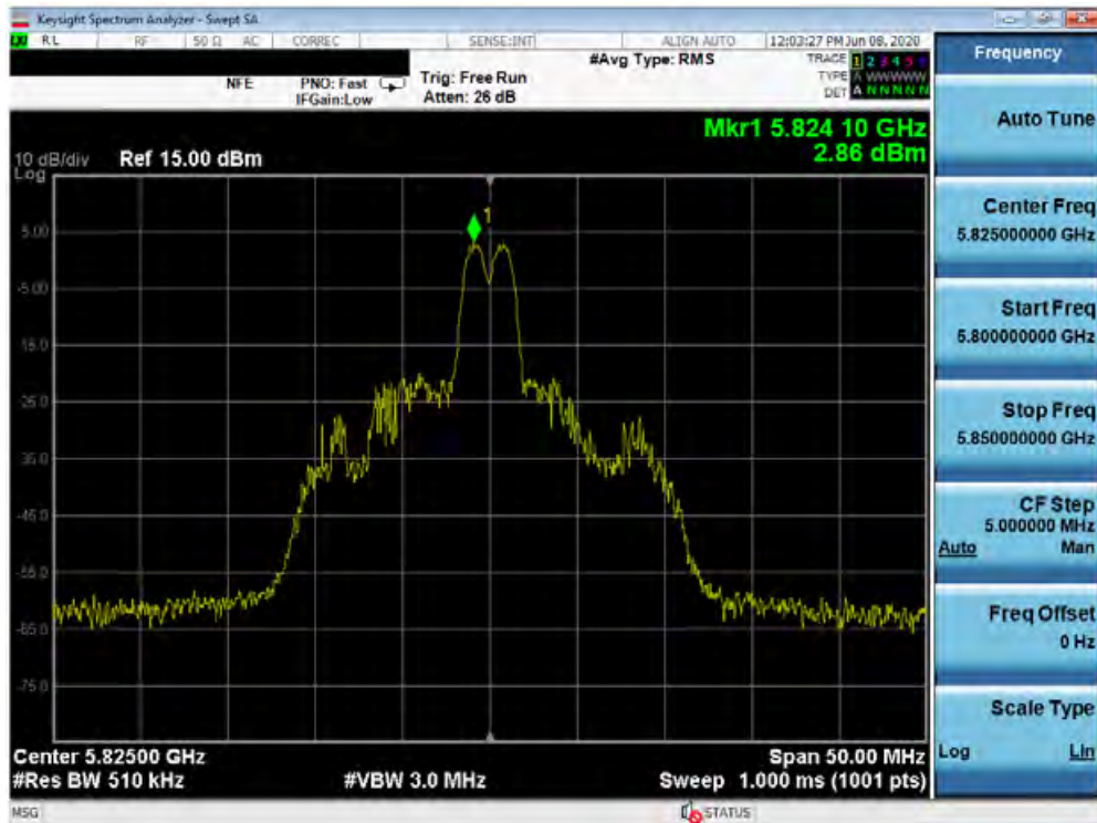
Plot 7-240. Power Spectral Density Plot MIMO ANT1 (20MHz BW 802.11ax – 26 Tones (UNII Band 3) – Ch. 165)
