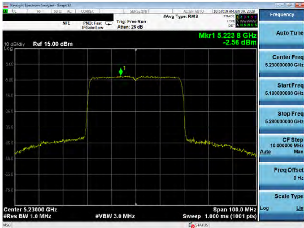
Plot 7-302. Power Spectral Density Plot MIMO ANT2 (40MHz BW 802.11ax – Full Tones (UNII Band 1) – Ch. 46)
