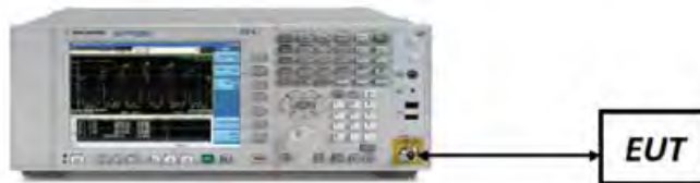
Figure 7-1. Test Instrument & Measurement Setup
