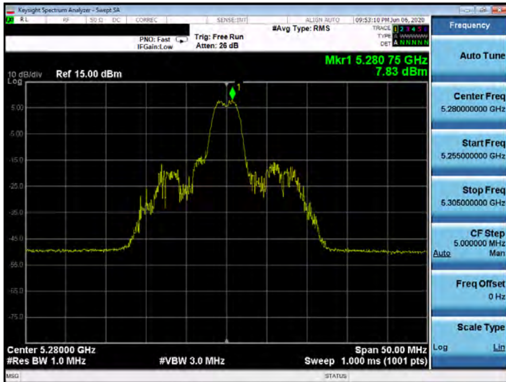
Plot 7-116. Power Spectral Density Plot SISO ANT1 (20MHz BW 802.11ax – 26 Tones (UNII Band 2A) – Ch. 56)
