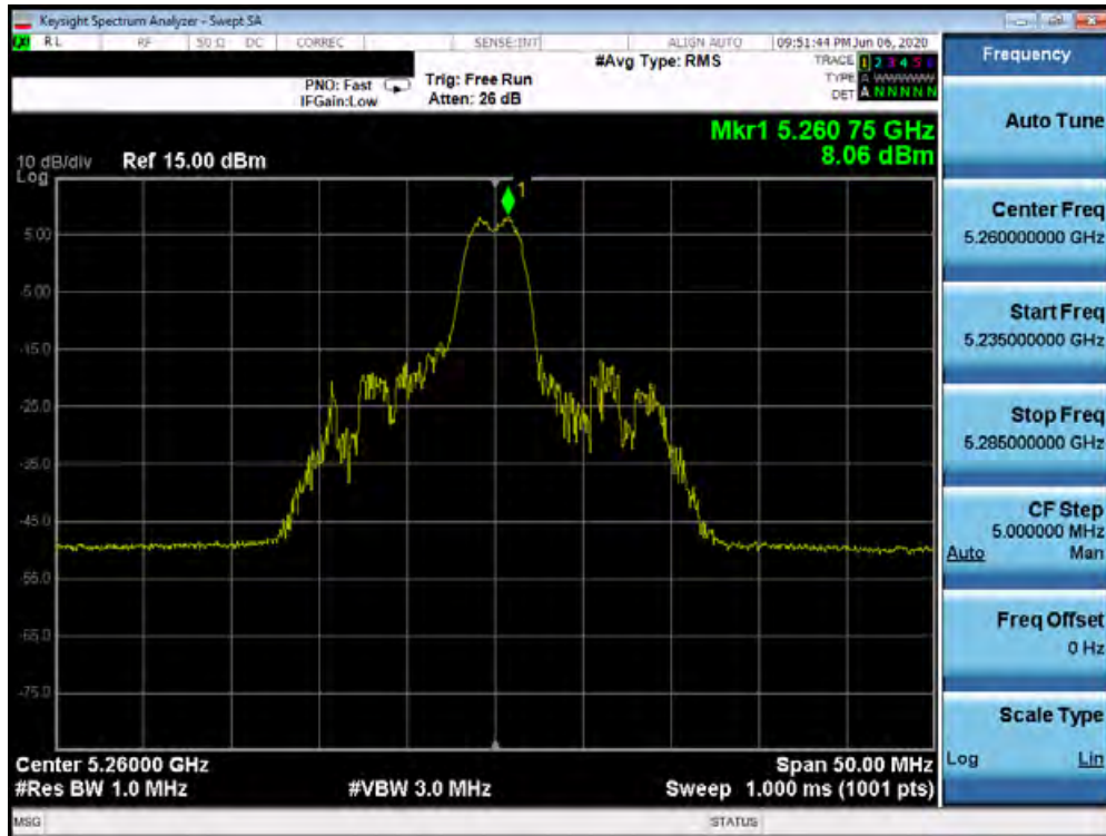
Plot 7-115. Power Spectral Density Plot SISO ANT1 (20MHz BW 802.11ax – 26 Tones (UNII Band 2A) – Ch. 52)
