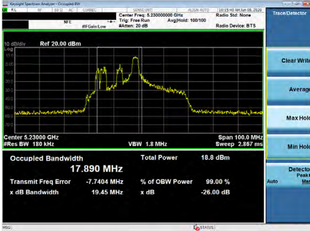
Plot 7-47. 26dB Bandwidth Plot SISO ANT2 (40MHz BW 802.11ax – 26 Tones (UNII Band 1) – Ch. 46)
