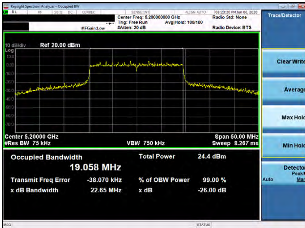
Plot 7-23. 26dB Bandwidth Plot SISO ANT1 (20MHz BW 802.11ax – 242 Tones (UNII Band 1) – Ch. 40)
