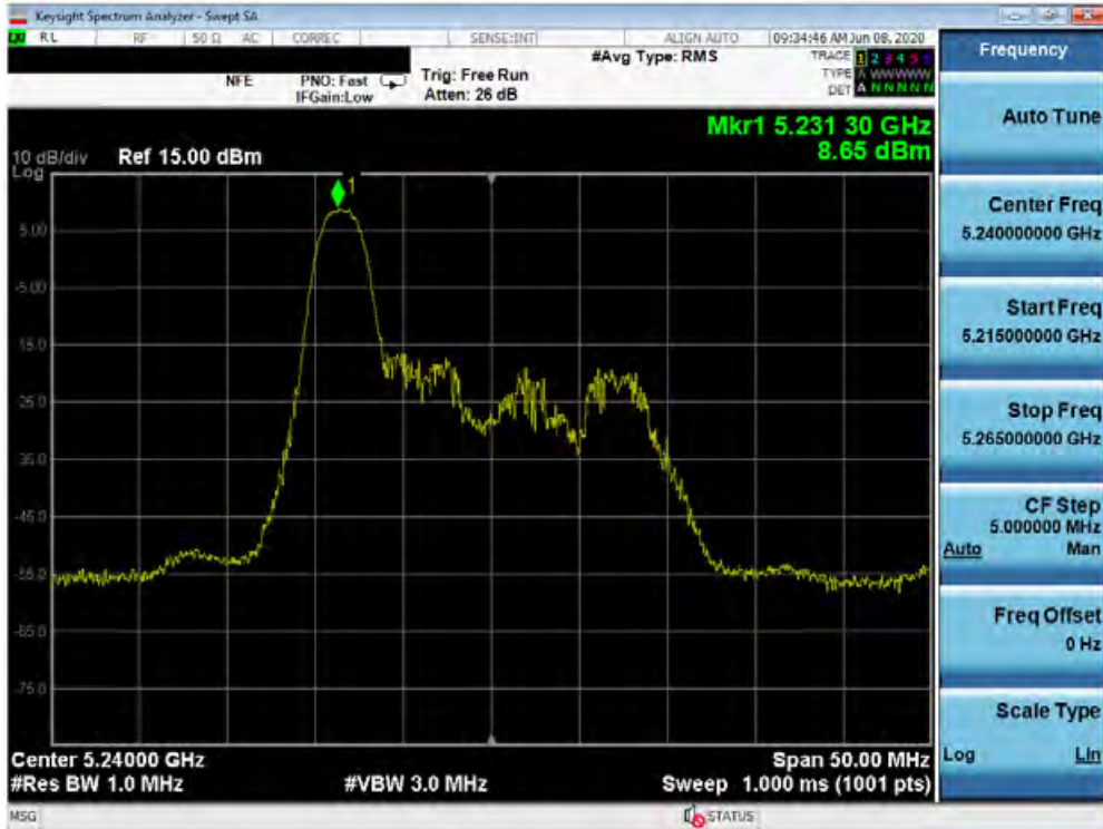
Plot 7-165. Power Spectral Density Plot SISO ANT2 (20MHz BW 802.11ax – 26 Tones (UNII Band 1) – Ch. 48)
