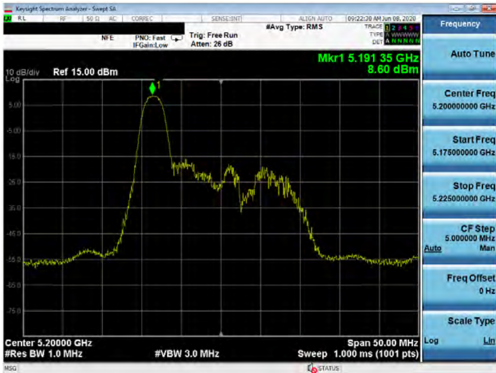
Plot 7-164. Power Spectral Density Plot SISO ANT2 (20MHz BW 802.11ax – 26 Tones (UNII Band 1) – Ch. 40)
