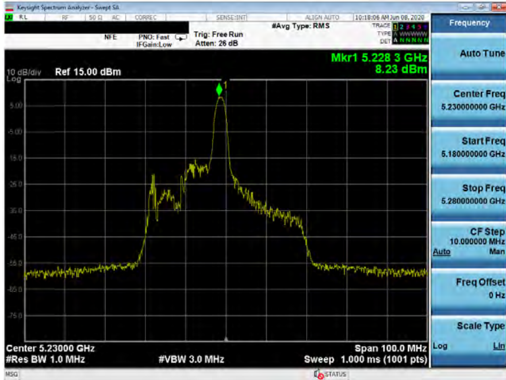
Plot 7-167. Power Spectral Density Plot SISO ANT2 (40MHz BW 802.11ax – 26 Tones (UNII Band 1) – Ch. 46)
