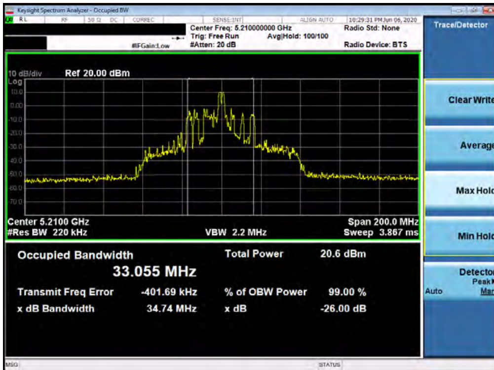
Plot 7-6. 26dB Bandwidth Plot SISO ANT1 (80MHz BW 802.11ax – 26 Tones (UNII Band 1) – Ch. 42)
