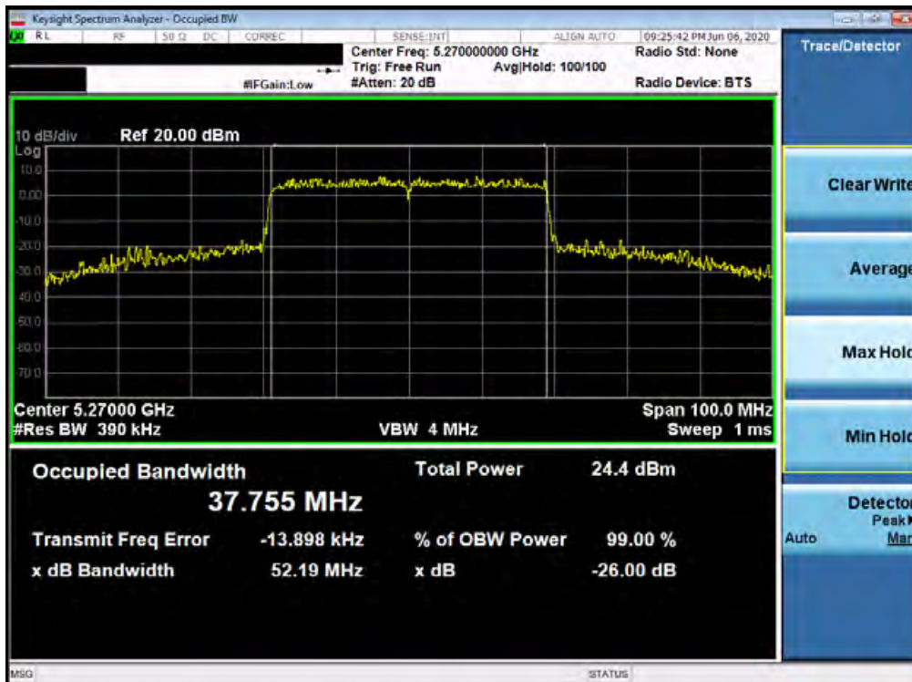
Plot 7-31. 26dB Bandwidth Plot SISO ANT1 (40MHz BW 802.11ax – 484 Tones (UNII Band 2A) – Ch. 54)
