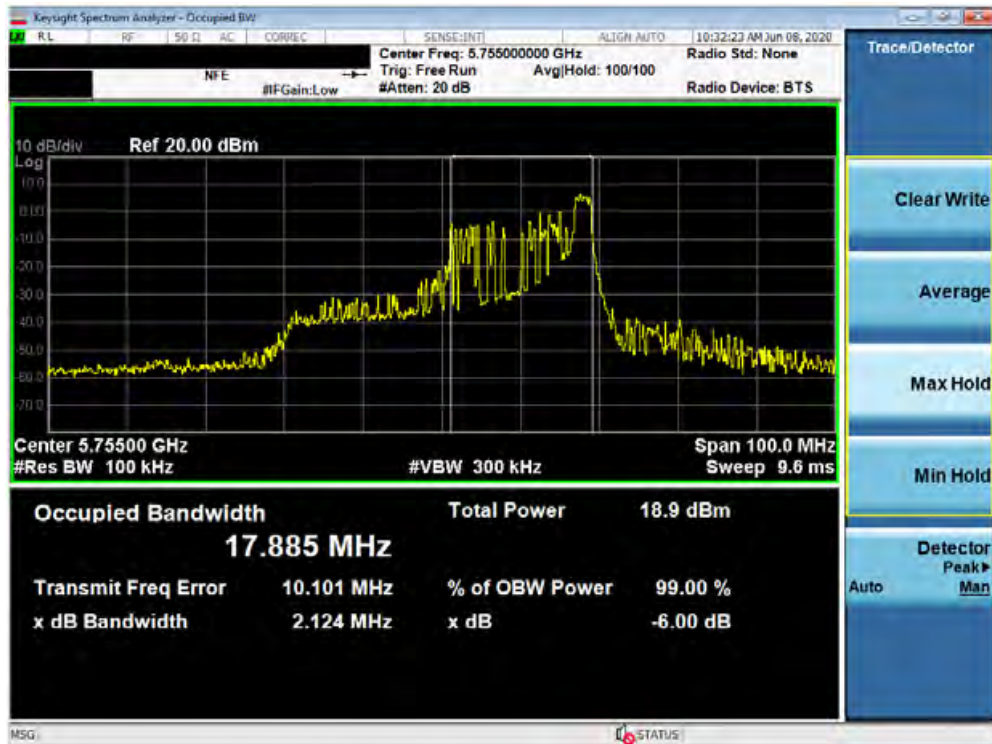
Plot 7-100. 6dB Bandwidth Plot SISO ANT2 (40MHz BW 802.11ax – 26 Tones (UNII Band 3) – Ch. 151)
