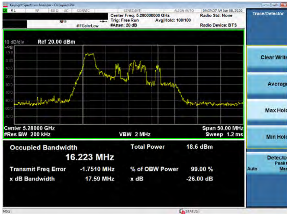
Plot 7-50. 26dB Bandwidth Plot SISO ANT2 (20MHz BW 802.11ax – 26 Tones (UNII Band 2A) – Ch. 56)
