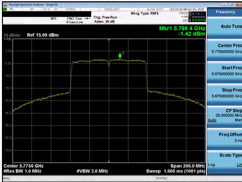
Plot 7-191. Power Spectral Density Plot SISO ANT1 (80MHz BW 802.11ac (UNII Band 3) – Ch. 155)
