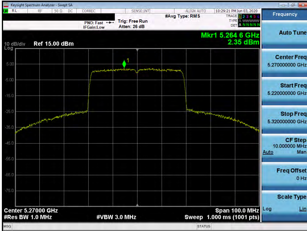
Plot 7-219. Power Spectral Density Plot SISO ANT2 (40MHz BW 802.11ax (UNII Band 2A) – Ch. 54)
