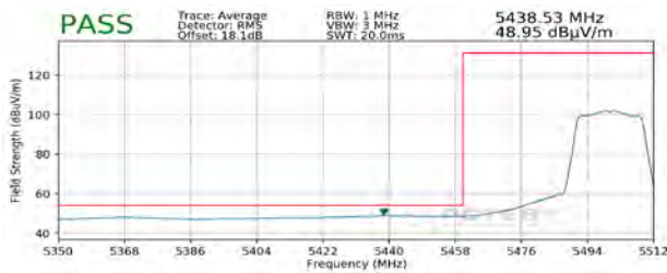
Plot 7-286. Radiated Lower Band Edge Plot SISO ANT1 (Average – UNII Band 2C)
