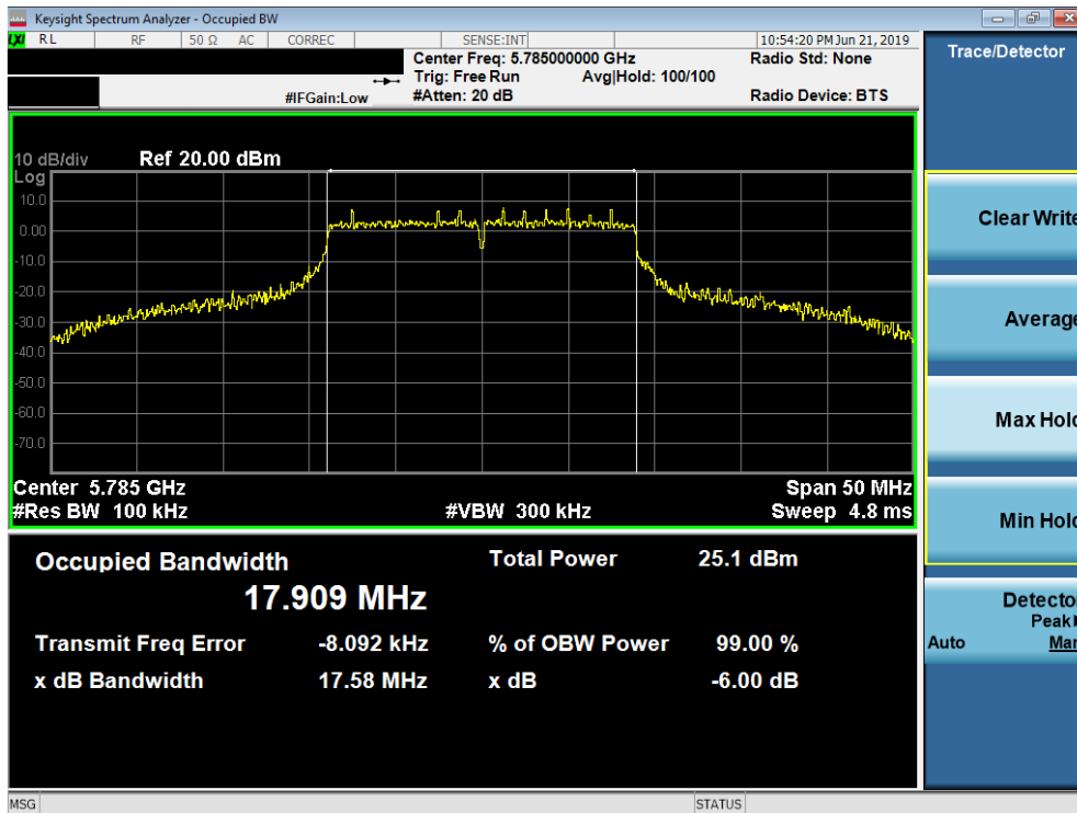
Plot 7-101. 6dB Bandwidth Plot SISO ANT1 (20MHz BW 802.11n (UNII Band 3) – Ch. 157)
