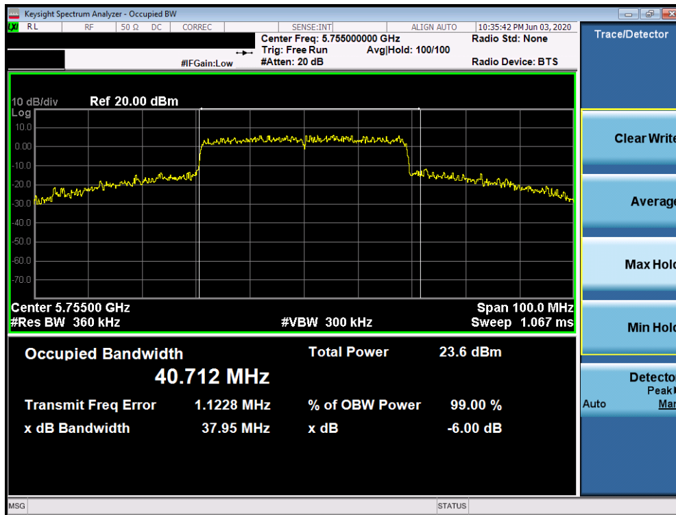
Plot 7-123. 6dB Bandwidth Plot SISO ANT2 (40MHz BW 802.11ax (UNII Band 3) – Ch. 151)
