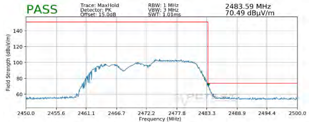
Plot 7-128. Radiated Restricted Upper Band Edge Measurement MIMO (Peak – 106 Tones)
