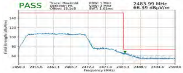
Plot 7-136. Radiated Restricted Upper Band Edge Measurement MIMO (Peak – 242 Tones)
