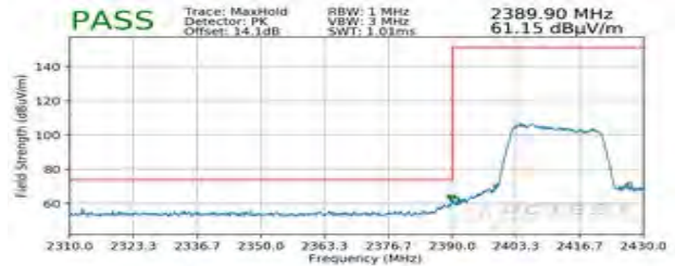
Plot 7-130. Radiated Restricted Lower Band Edge Measurement MIMO (Peak – 242 Tones)
