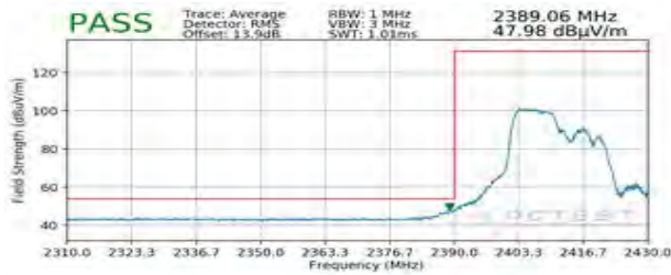
Plot 7-121. Radiated Restricted Lower Band Edge Measurement MIMO (Average – 106 Tones)
