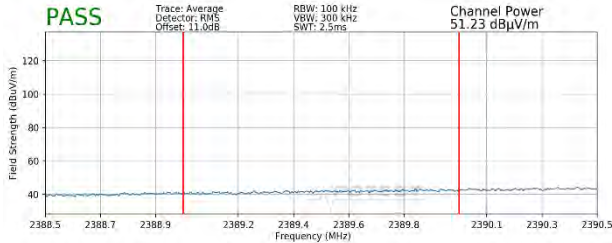
Plot 7-89. Radiated Restricted Lower Band Edge Measurement SISO ANT1 (Average – 242 Tones)
