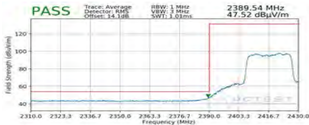
Plot 7-131. Radiated Restricted Lower Band Edge Measurement MIMO (Average – 242 Tones)
