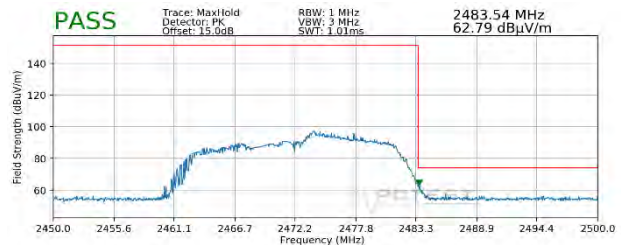
Plot 7-108. Radiated Restricted Upper Band Edge Measurement SISO ANT2 (Peak – 106 Tones)
