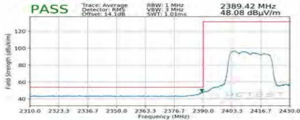
Plot 7-129. Radiated Restricted Lower Band Edge Measurement MIMO (Average – 242 Tones)
