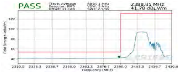
Plot 7-101. Radiated Restricted Lower Band Edge Measurement SISO ANT2 (Average – 106 Tones)
