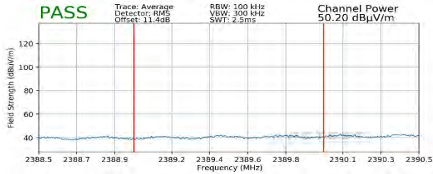
Plot 7-109. Radiated Restricted Lower Band Edge Measurement SISO ANT2 (Average – 242 Tones)
