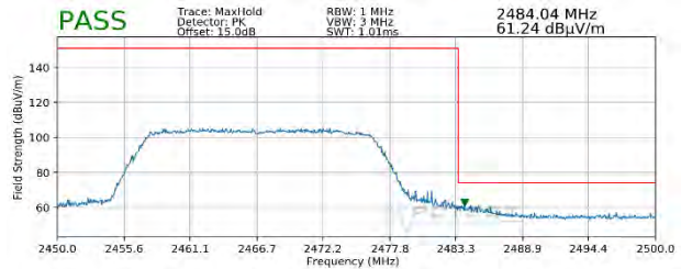
Plot 7-138. Radiated Restricted Upper Band Edge Measurement MIMO (Peak – 242 Tones)
