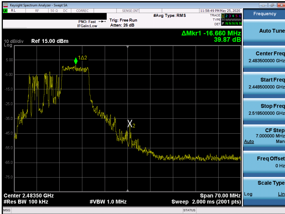
Plot 7-30. Band Edge Plot SISO ANT2 (802.11ax OFDMA – 106 Tones – Ch. 11)
