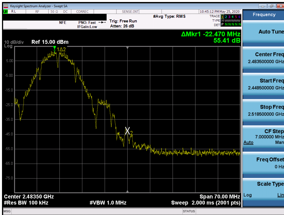
Plot 7-70. Band Edge Plot SISO ANT2 (802.11b – Ch. 11)
