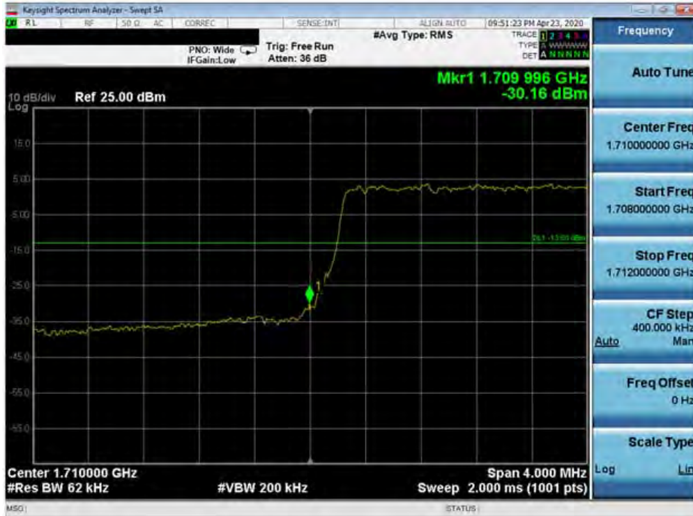
Plot 7-132. Lower Band Edge Plot (Band 4 - 5.0MHz QPSK - Full RB Configuration)
