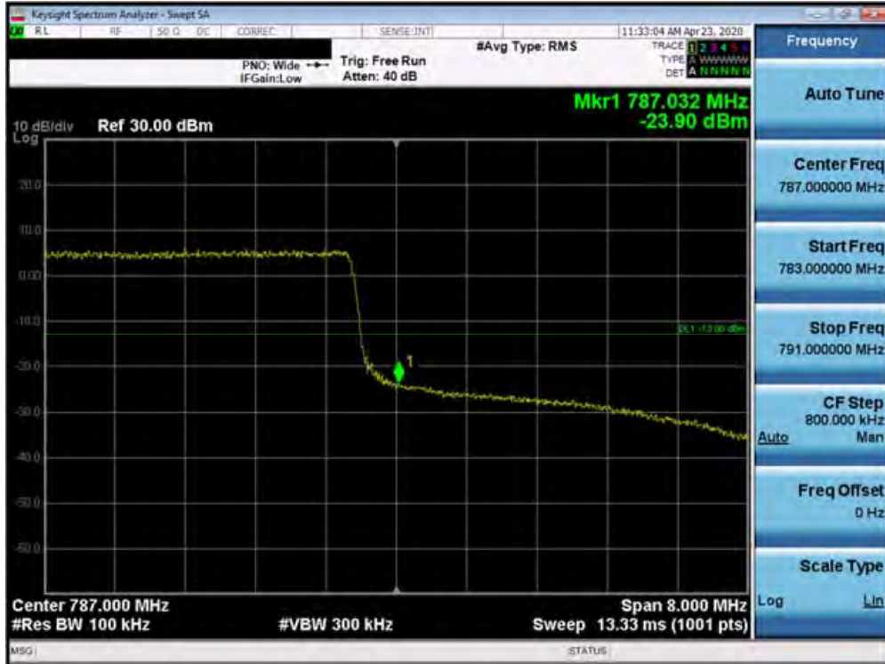
Plot 7-114. Upper Band Edge Plot (Band 13 - 10.0MHz QPSK - Full RB Configuration)
