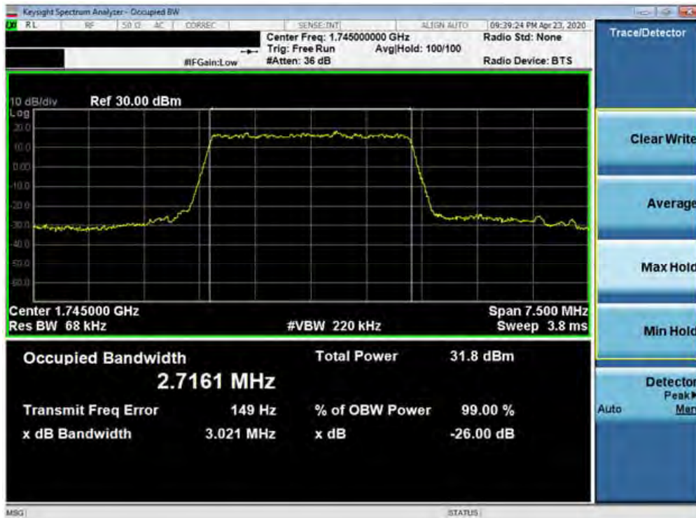
Plot 7-34. Occupied Bandwidth Plot (Band 4 - 3.0MHz QPSK - Full RB Configuration)
