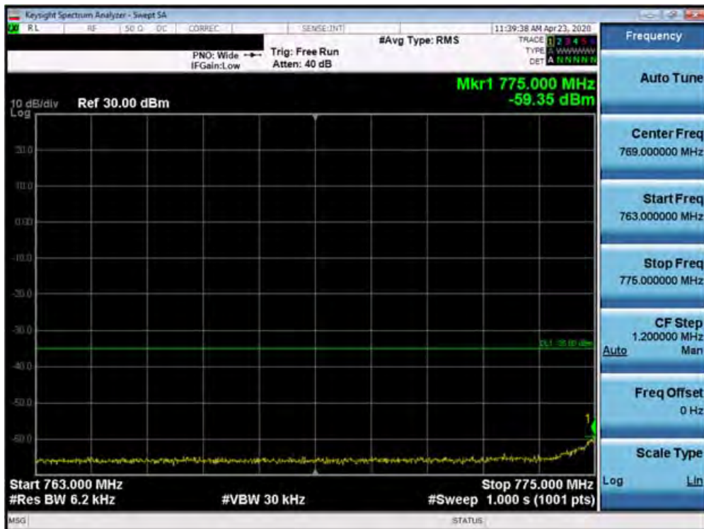
Plot 7-109. Lower Extended Band Edge Plot (Band 13 - 5.0MHz QPSK - Full RB Configuration)
