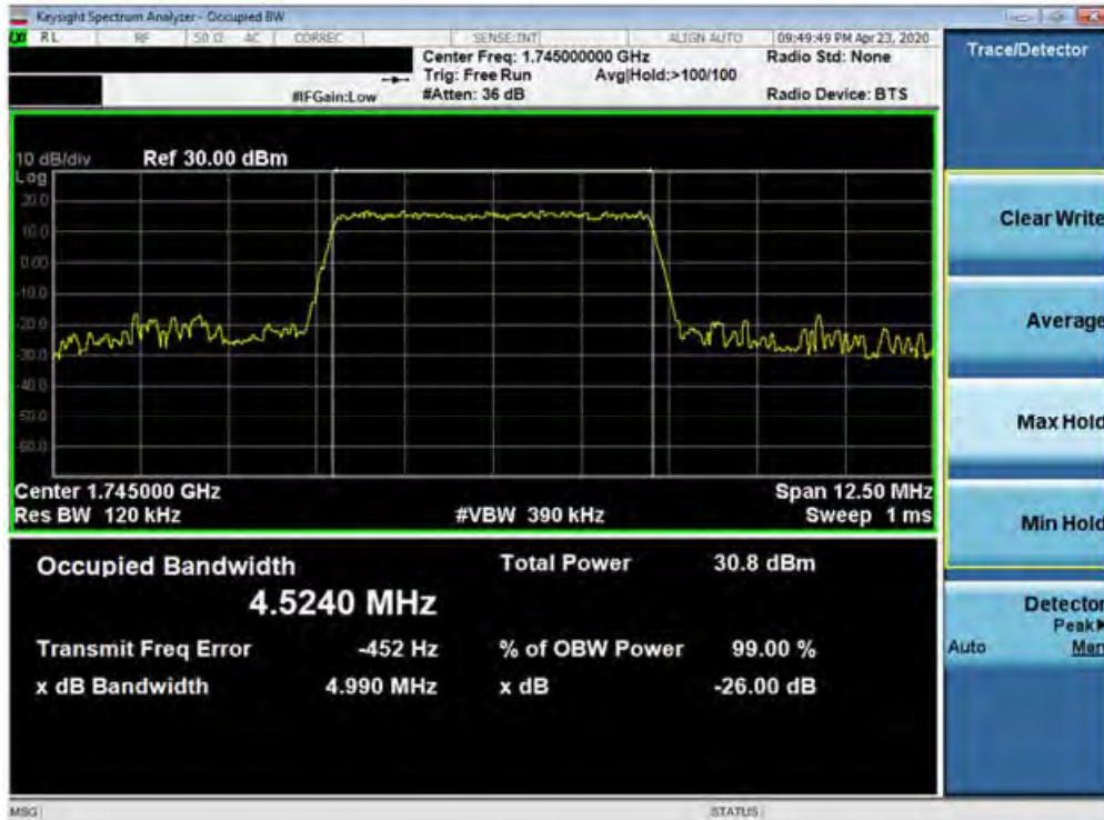
Plot 7-38. Occupied Bandwidth Plot (Band 4 - 5.0MHz 16-QAM - Full RB Configuration)
