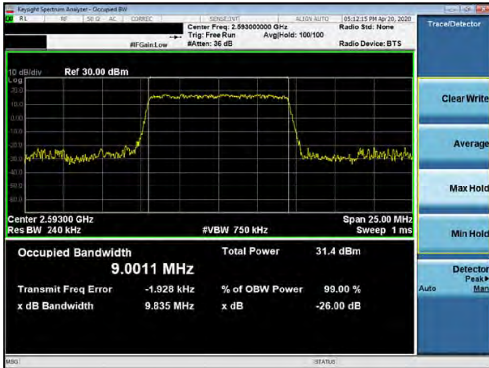
Plot 7-52. Occupied Bandwidth Plot (Band 41 (PC3) - 10.0MHz QPSK - Full RB Configuration)
