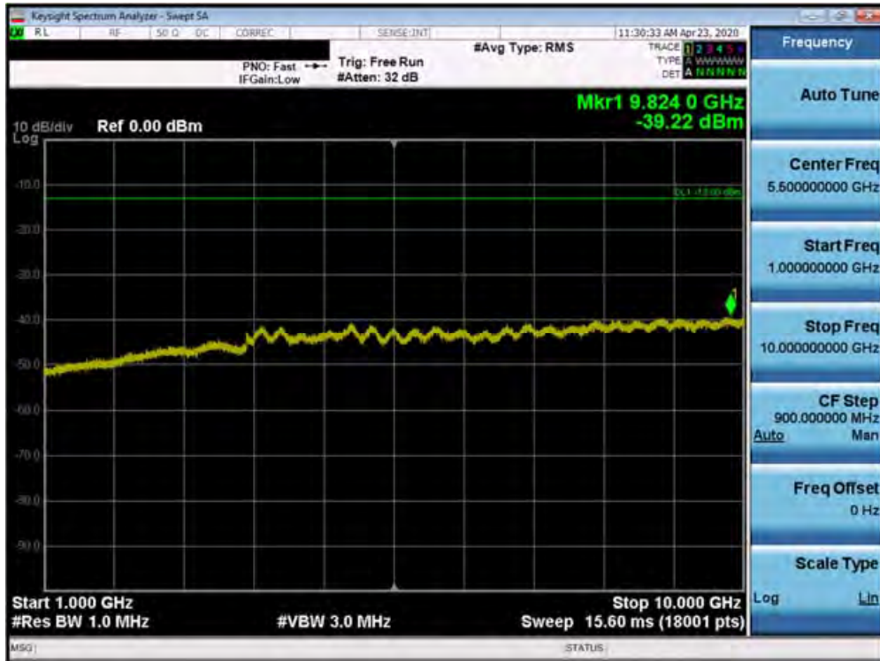
Plot 7-72. Conducted Spurious Plot (Band 13 - 10.0MHz QPSK - RB Size 1, RB Offset 0)
