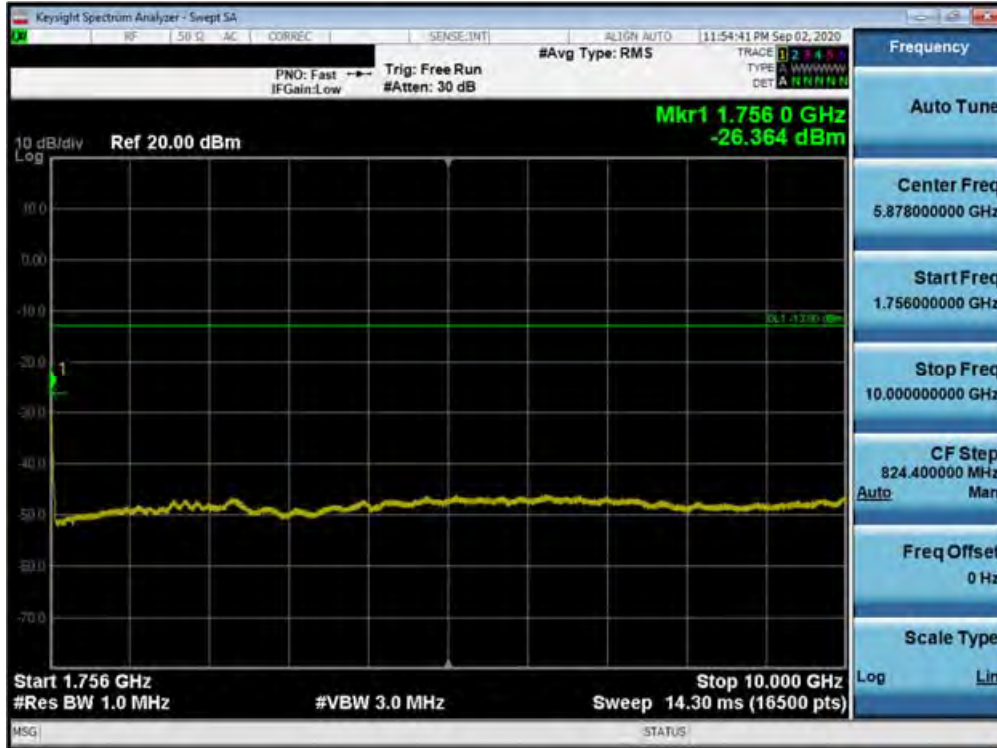
Plot 7-86. Conducted Spurious Plot (Band 4 - 20.0MHz QPSK - RB Size 1, RB Offset 0 - Mid Channel)
