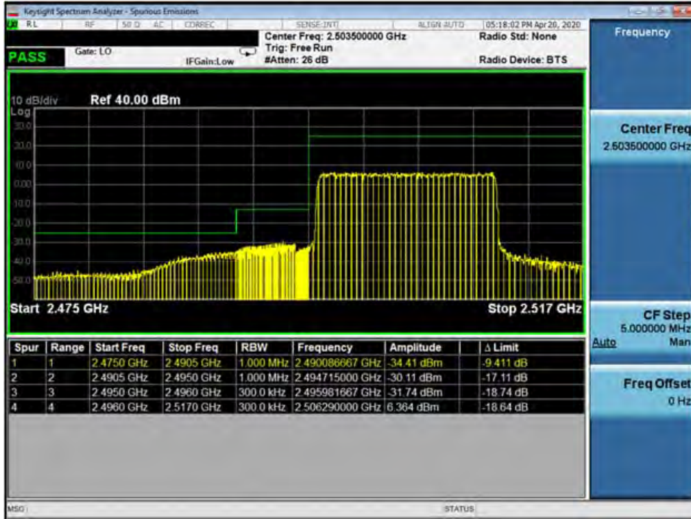
Plot 7-152. Lower ACP Plot at 2496 MHz (Band 41 PC3- 15.0MHz QPSK - Full RB Configuration)
