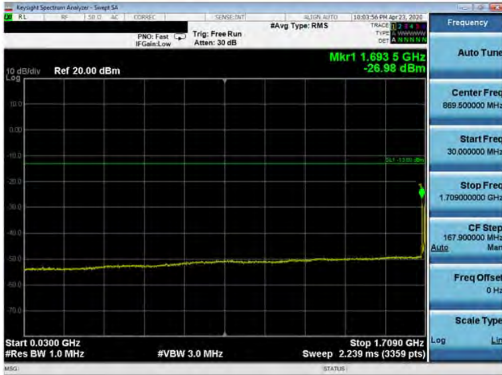
Plot 7-82. Conducted Spurious Plot (Band 4 - 20.0MHz QPSK - RB Size 1, RB Offset 0 - Low Channel)
