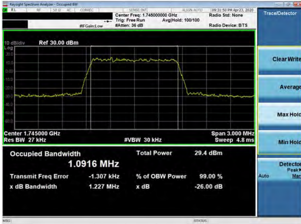
Plot 7-33. Occupied Bandwidth Plot (Band 4 - 1.4MHz 64-QAM - Full RB Configuration)
