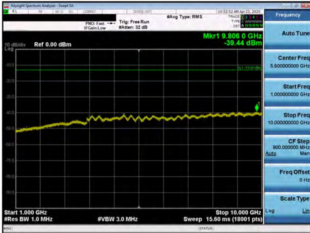
Plot 7-63. Conducted Spurious Plot (Band 12 - 10.0MHz QPSK - RB Size 1, RB Offset 0 - Low Channel)
