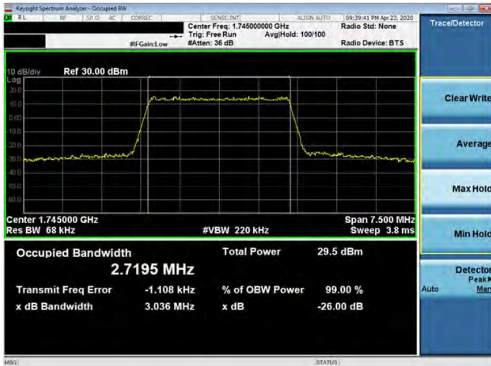
Plot 7-36. Occupied Bandwidth Plot (Band 4 - 3.0MHz 64-QAM - Full RB Configuration)
