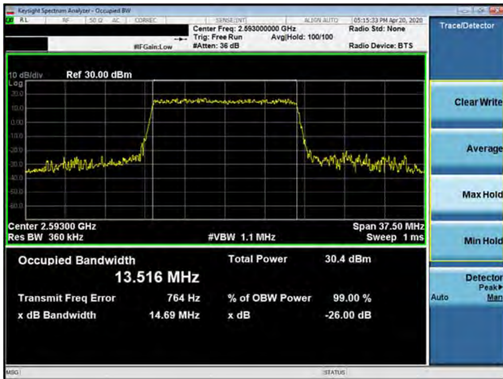
Plot 7-56. Occupied Bandwidth Plot (Band 41 (PC3) - 15.0MHz 16-QAM - Full RB Configuration)
