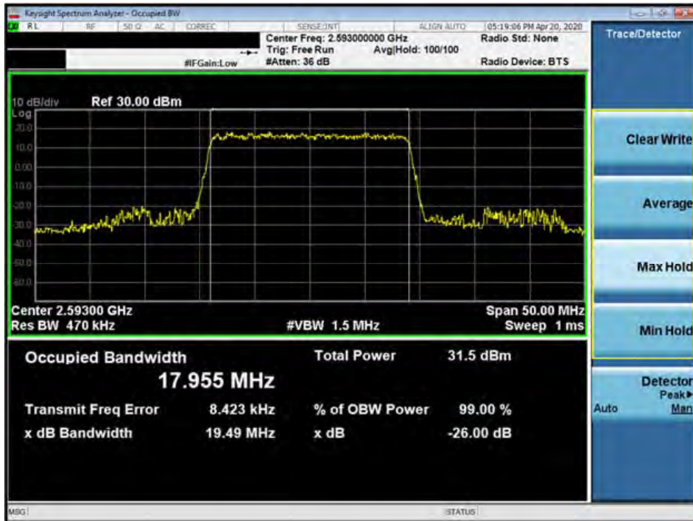
Plot 7-58. Occupied Bandwidth Plot (Band 41 (PC3) - 20.0MHz QPSK - Full RB Configuration)
