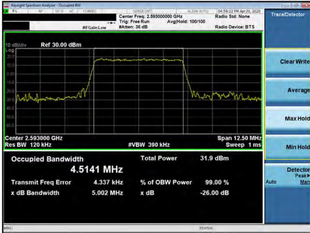
Plot 7-49. Occupied Bandwidth Plot (Band 41 (PC3) - 5.0MHz QPSK - Full RB Configuration)
