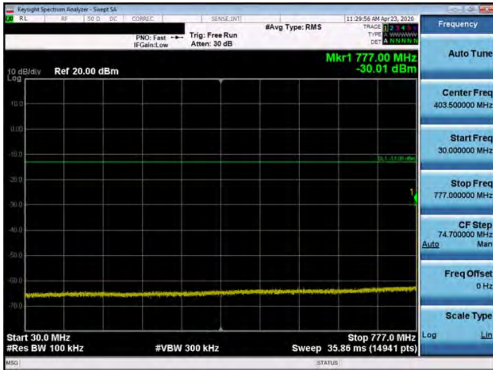
Plot 7-70. Conducted Spurious Plot (Band 13 - 10.0MHz QPSK - RB Size 1, RB Offset 0)
