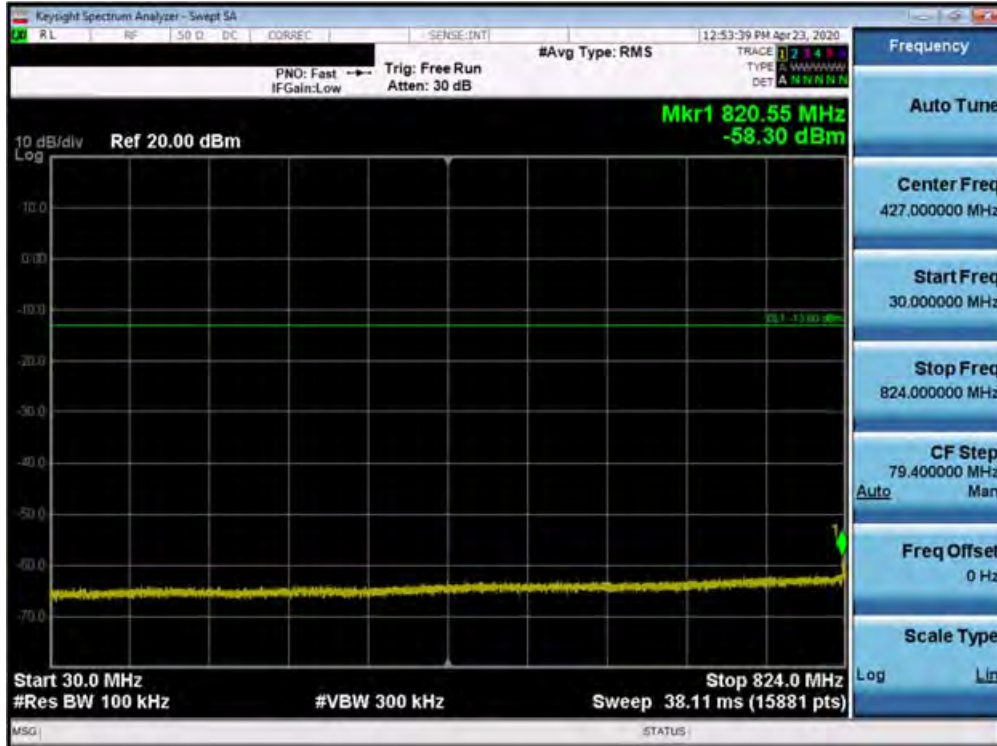
Plot 7-79. Conducted Spurious Plot (Band 5 - 10.0MHz QPSK - RB Size 1, RB Offset 0 - High Channel)
