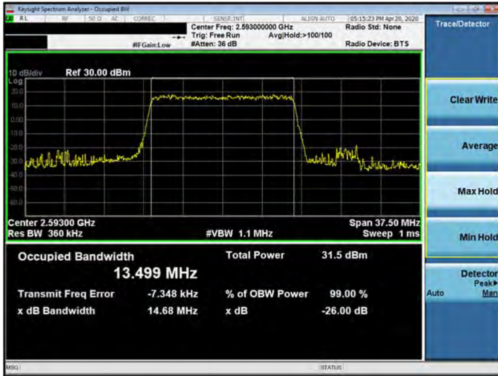
Plot 7-55. Occupied Bandwidth Plot (Band 41 (PC3) - 15.0MHz QPSK - Full RB Configuration)
