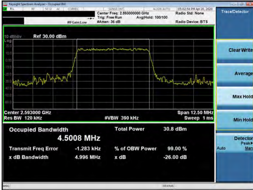
Plot 7-51. Occupied Bandwidth Plot (Band 41 (PC3) - 5.0MHz 64-QAM - Full RB Configuration)
