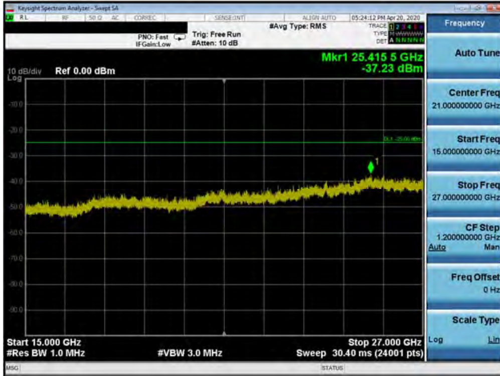
Plot 7-93. Conducted Spurious Plot (Band 41 PC3 - 20.0MHz QPSK - RB Size 1, RB Offset 0 - Low Channel)
