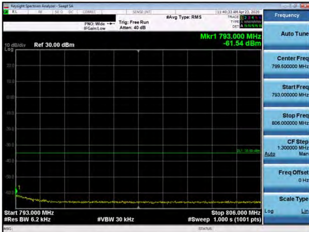
Plot 7-115. Upper Extended Band Edge Plot (Band 13 - 10.0MHz QPSK - Full RB Configuration)
