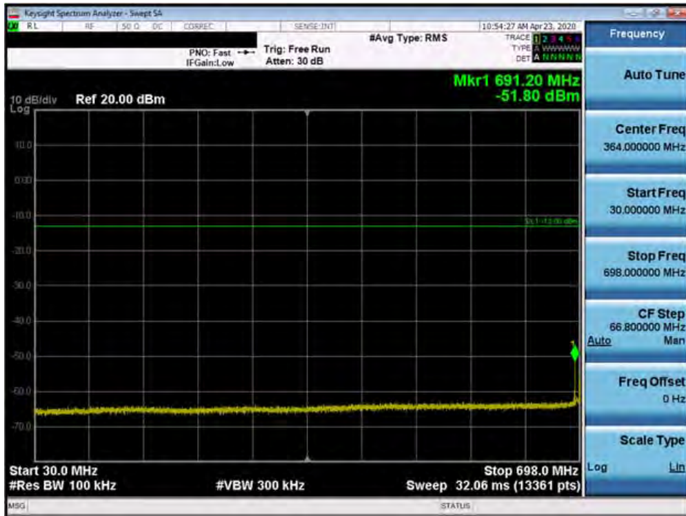
Plot 7-67. Conducted Spurious Plot (Band 12 - 10.0MHz QPSK - RB Size 1, RB Offset 0 - High Channel)
