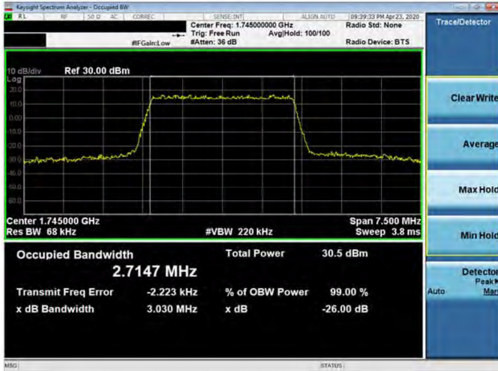
Plot 7-35. Occupied Bandwidth Plot (Band 4 - 3.0MHz 16-QAM - Full RB Configuration)
