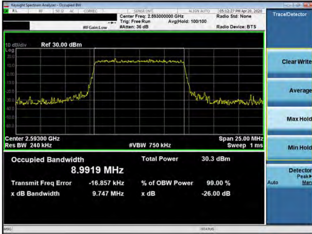
Plot 7-53. Occupied Bandwidth Plot (Band 41 (PC3) - 10.0MHz 16-QAM - Full RB Configuration)
