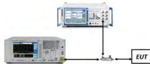
Figure 7-1. Test Instrument & Measurement Setup
