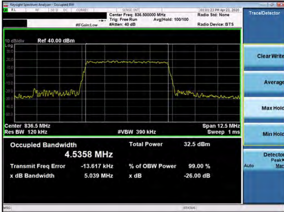
Plot 7-25. Occupied Bandwidth Plot (Band 5 - 5.0MHz QPSK - Full RB Configuration)
