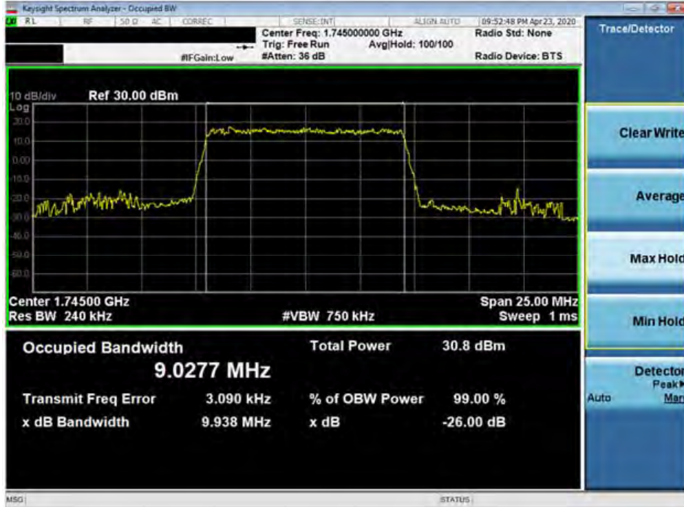
Plot 7-41. Occupied Bandwidth Plot (Band 4 - 10.0MHz 16-QAM - Full RB Configuration)
