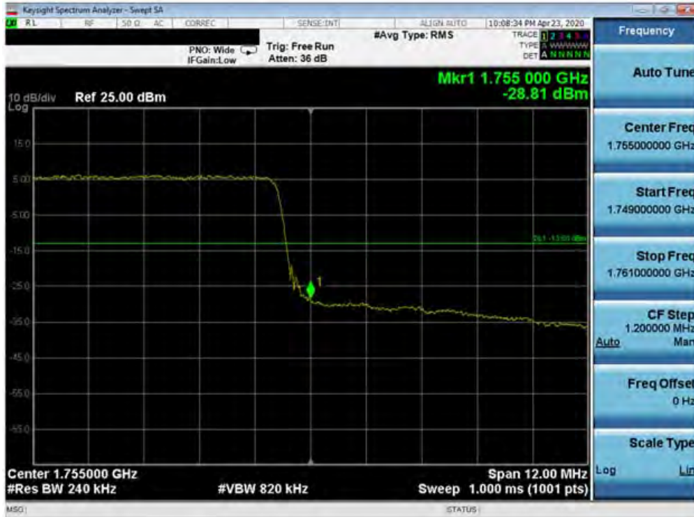
Plot 7-142. Upper Band Edge Plot (Band 4 - 15.0MHz QPSK - Full RB Configuration)
