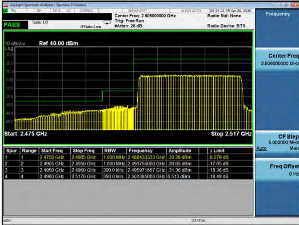
Plot 7-154. Lower ACP Plot at 2496 MHz (Band 41 PC3 - 20.0MHz QPSK - Full RB Configuration)
