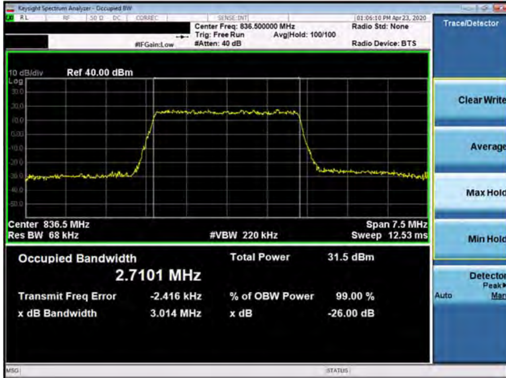
Plot 7-23. Occupied Bandwidth Plot (Band 5 - 3.0MHz 16-QAM - Full RB Configuration)
