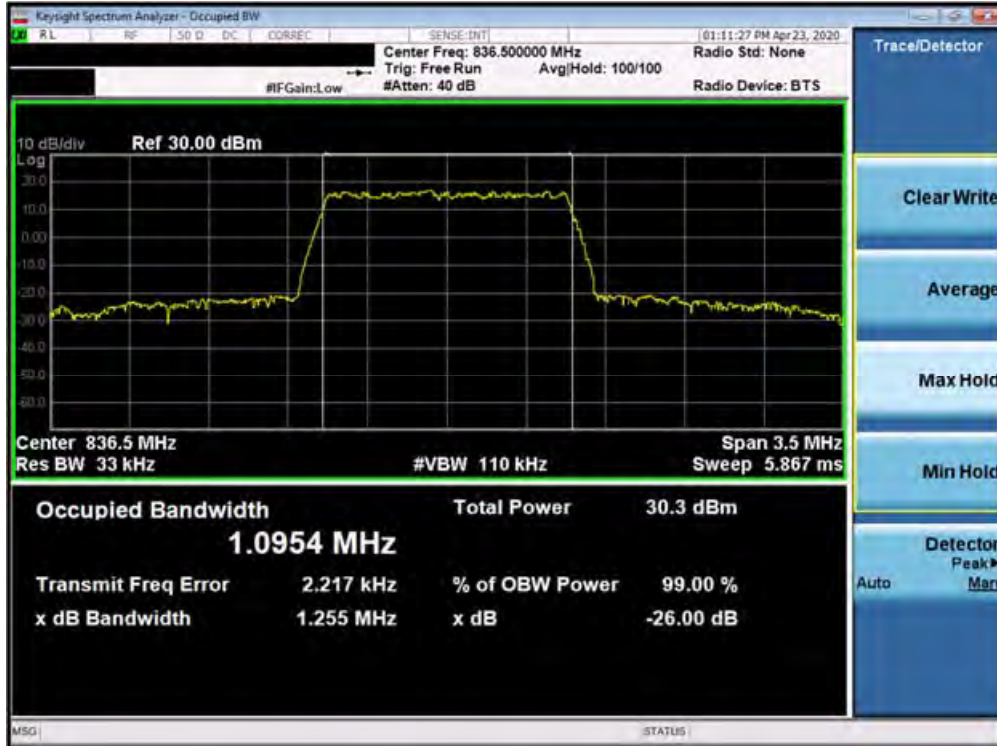
Plot 7-21. Occupied Bandwidth Plot (Band 5 - 1.4MHz 64-QAM - Full RB Configuration)
