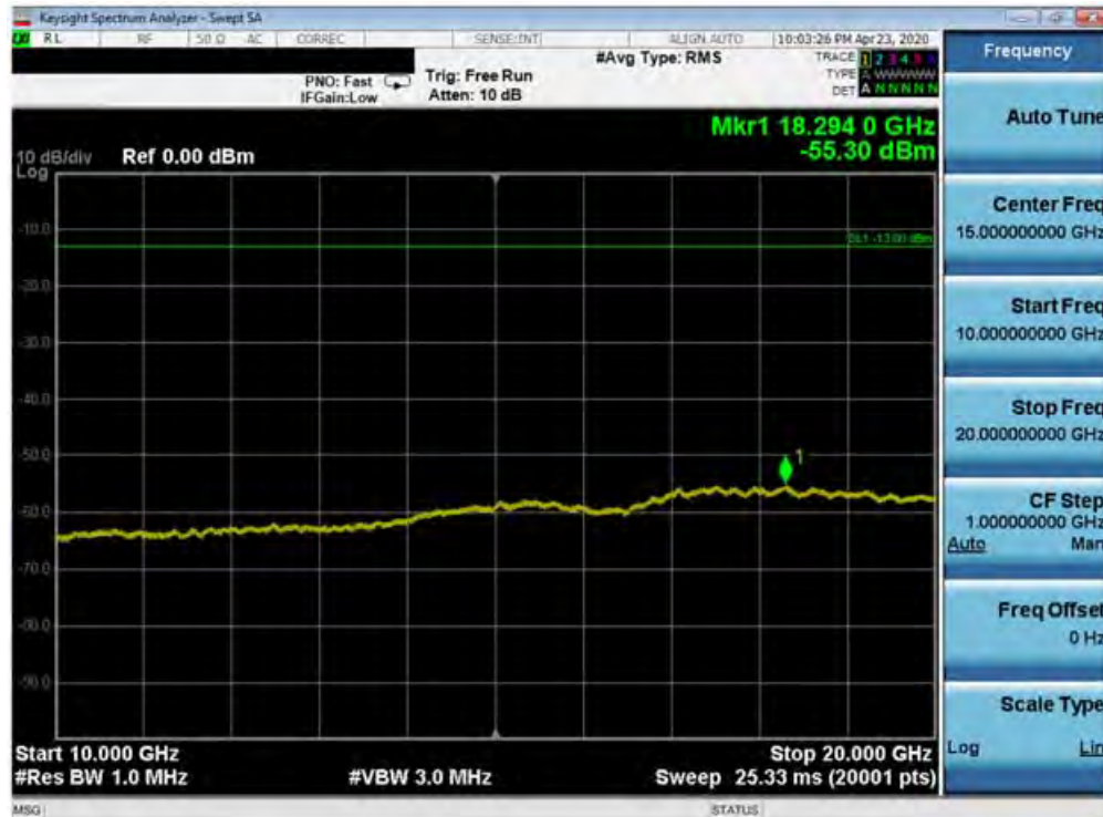
Plot 7-87. Conducted Spurious Plot (Band 4 - 20.0MHz QPSK - RB Size 1, RB Offset 0 - Mid Channel)
