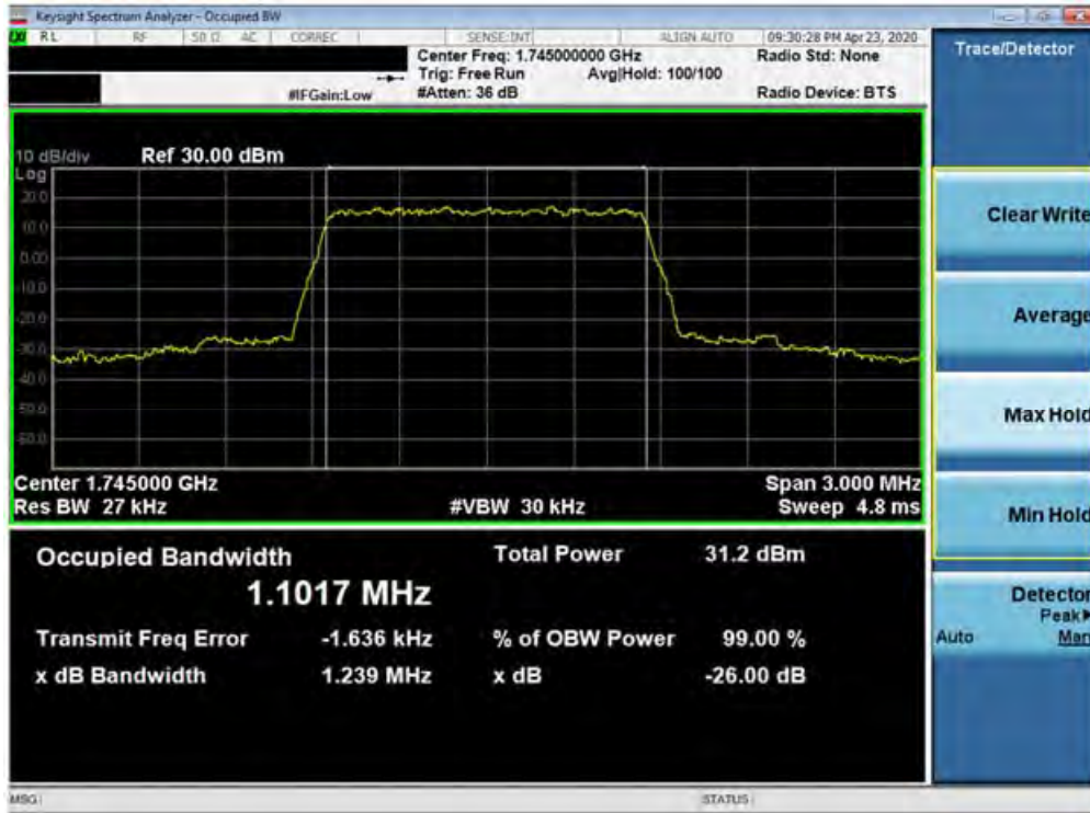
Plot 7-31. Occupied Bandwidth Plot (Band 4 - 1.4MHz QPSK - Full RB Configuration)
