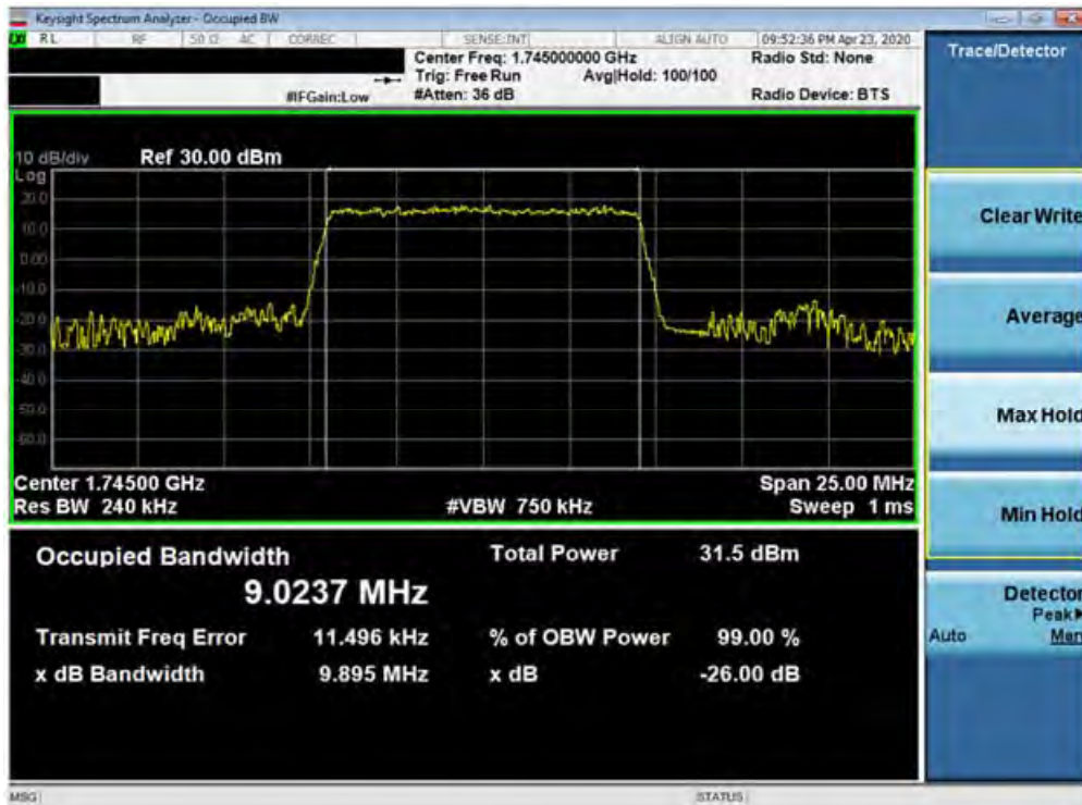
Plot 7-40. Occupied Bandwidth Plot (Band 4 - 10.0MHz QPSK - Full RB Configuration)
