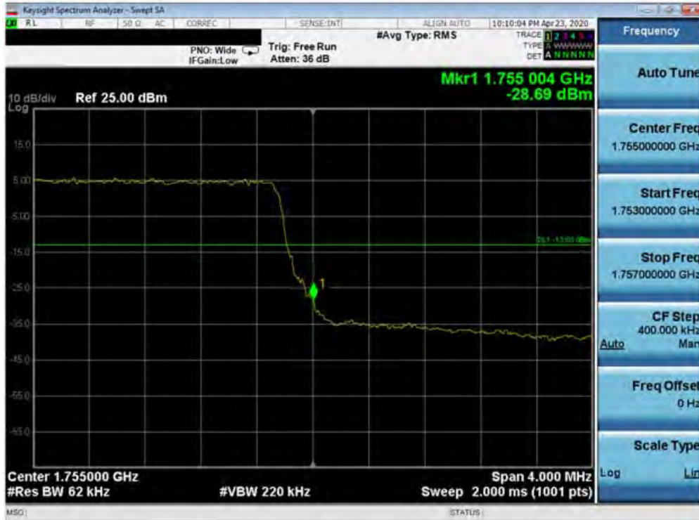
Plot 7-134. Upper Band Edge Plot (Band 4 - 5.0MHz QPSK - Full RB Configuration)
