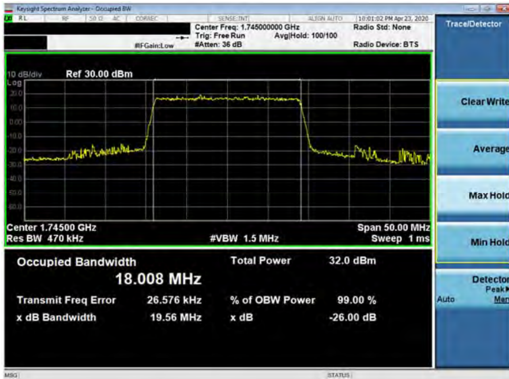
Plot 7-46. Occupied Bandwidth Plot (Band 4 - 20.0MHz QPSK - Full RB Configuration)
