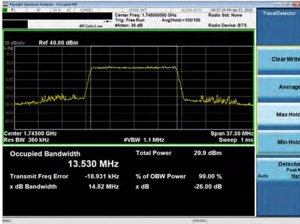
Plot 7-45. Occupied Bandwidth Plot (Band 4 - 15.0MHz 64-QAM - Full RB Configuration)
