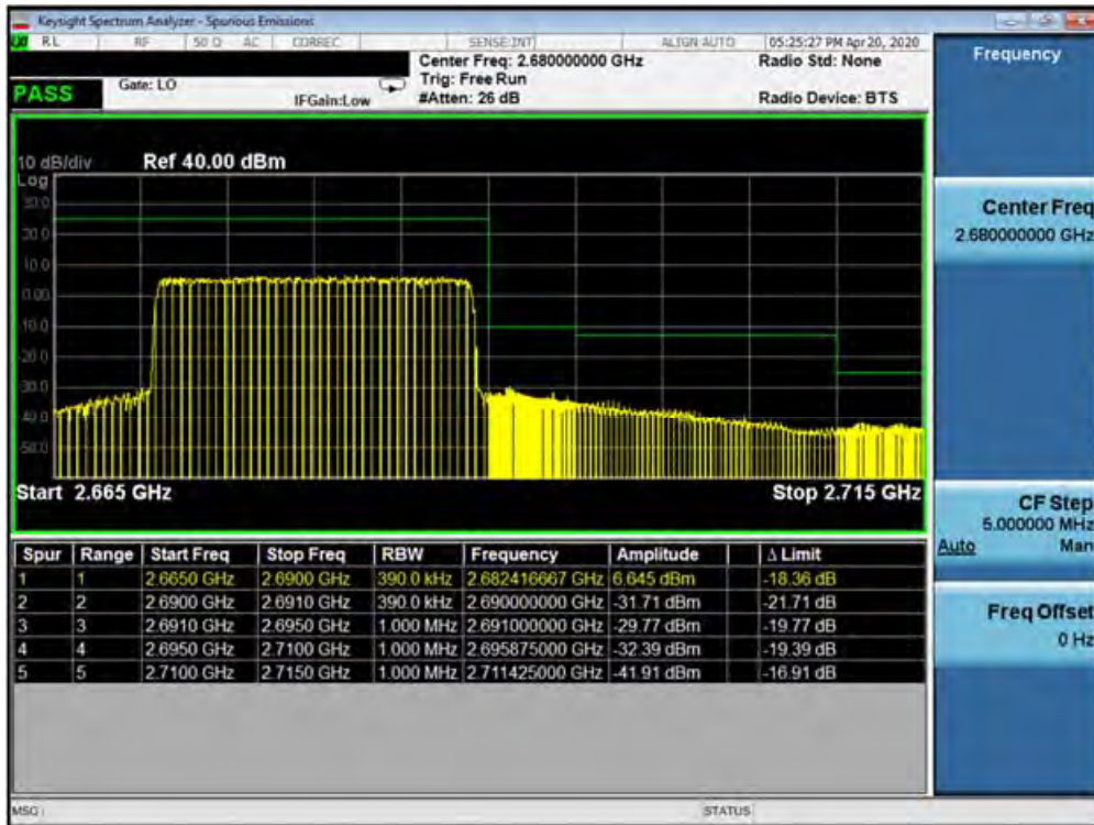
Plot 7-155. Upper ACP Plot (Band 41 PC3 - 20.0MHz QPSK - Full RB Configuration)
