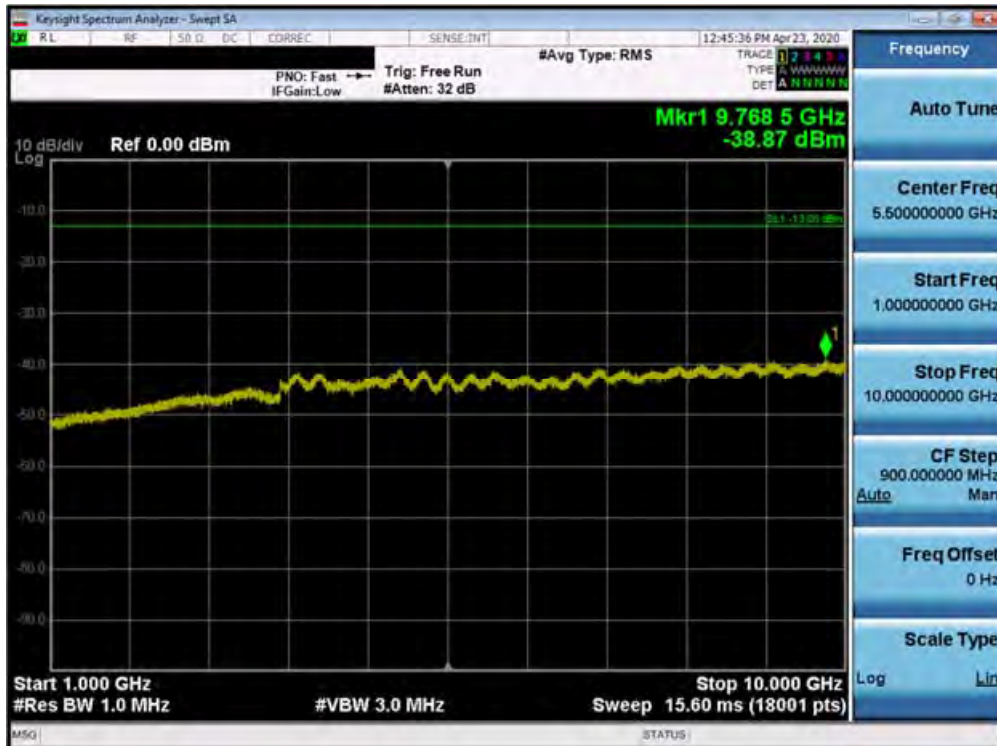
Plot 7-78. Conducted Spurious Plot (Band 5 - 10.0MHz QPSK - RB Size 1, RB Offset 0 - Mid Channel)
