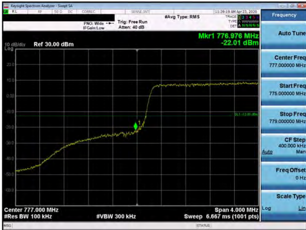
Plot 7-108. Lower Band Edge Plot (Band 13 - 5.0MHz QPSK - Full RB Configuration)
