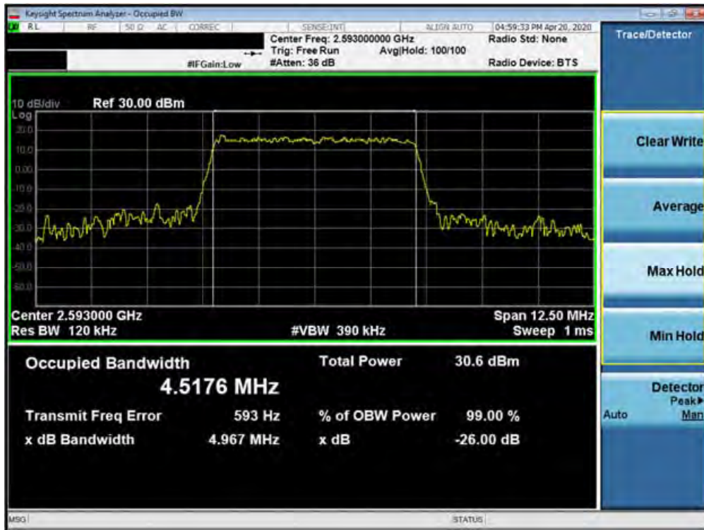
Plot 7-50. Occupied Bandwidth Plot (Band 41 (PC3) - 5.0MHz 16-QAM - Full RB Configuration)
