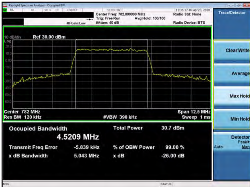
Plot 7-14. Occupied Bandwidth Plot (Band 13 - 5.0MHz 16-QAM - Full RB Configuration)
