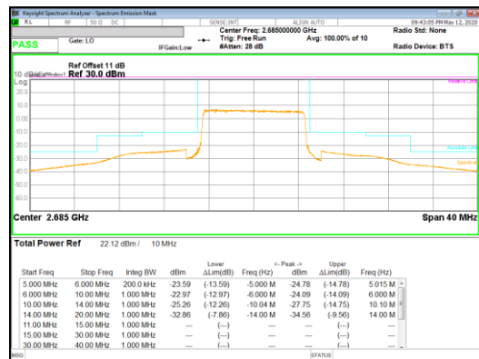
16QAM High channel FRB
